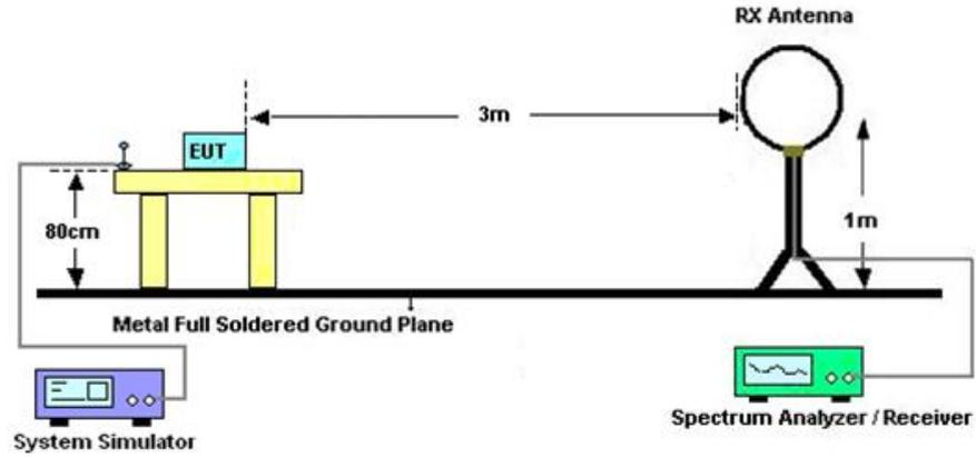
For radiated emissions from 30MHz to 1GHz
