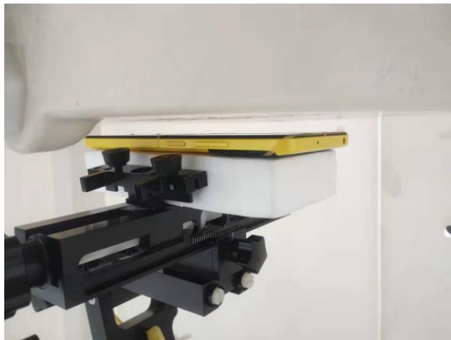
Front, Test Separation 10 mm
