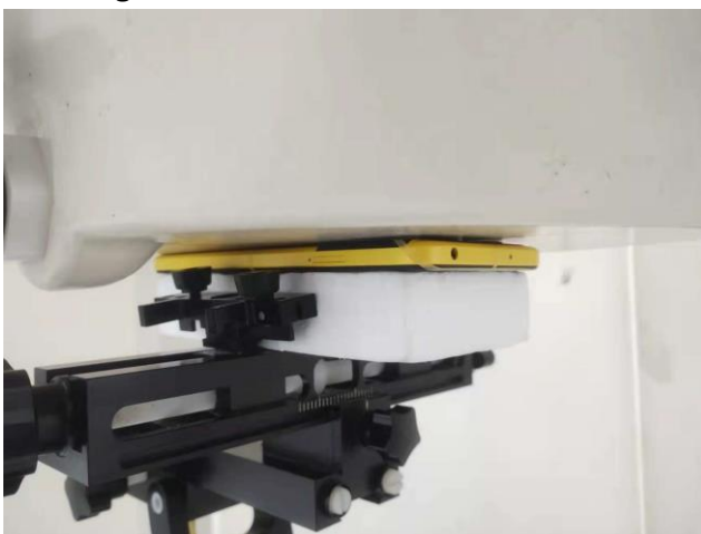
Back, Test Separation 0 mm
