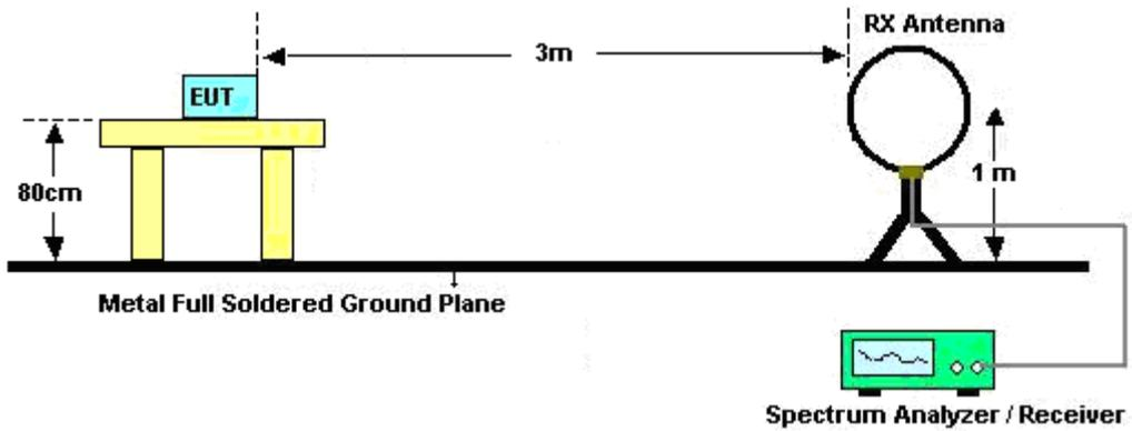
For radiated test from 30MHz to 1GHz
