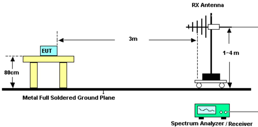
For radiated test above 1GHz
