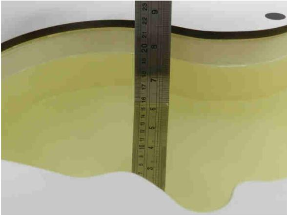
Fig 11.1 Photo of Liquid Height for Head SAR
