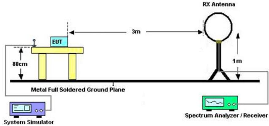
For radiated emissions from 30MHz to 1GHz
