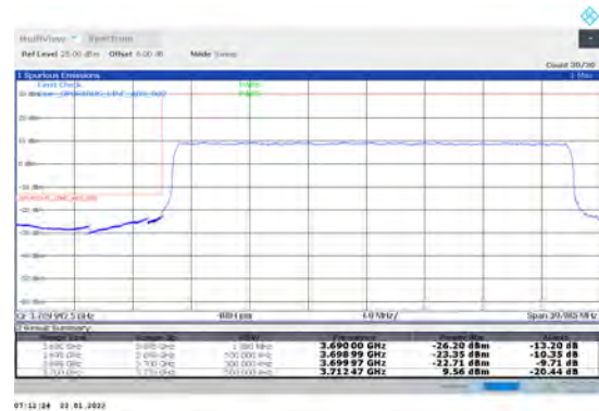
1-N78-3700-3800-PC3-30-30-L-3-DFT-PI2BPSK-O uter_Full-75@0-Ant1-PASS-see graph
