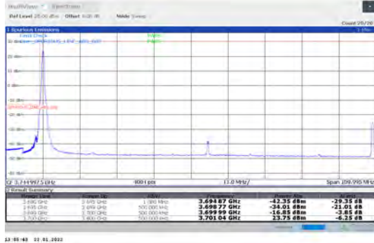
1-N78-3700-3800-PC2-30-100-L-4-CP-QPSK-Edge_1 RB_Left-1@0-Ant1-PASS-see graph
