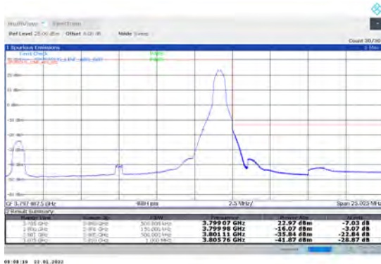
1-N78-3700-3800-PC2-30-15-H-2-DFT-PI2BPSK-Edge _1RB_Right-1@37-Ant1-PASS-see graph
