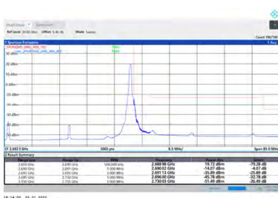
1-N41-PC3-30-40-H-2-DFT-PI2BPSK-Edge_1RB_Ri ght1@105-Ant1-PASS-see graph
