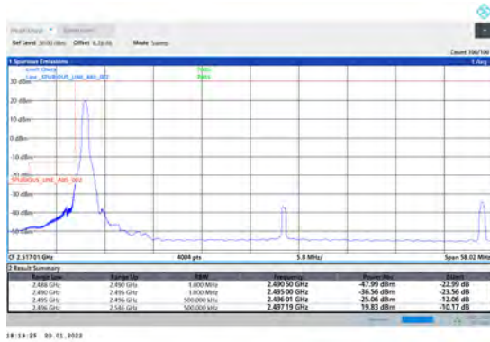
1-N41-PC3-30-50-L-1-DFT-PI2BPSK-Edge_1RB_Lef t-1@0-Ant1-PASS-see graph
