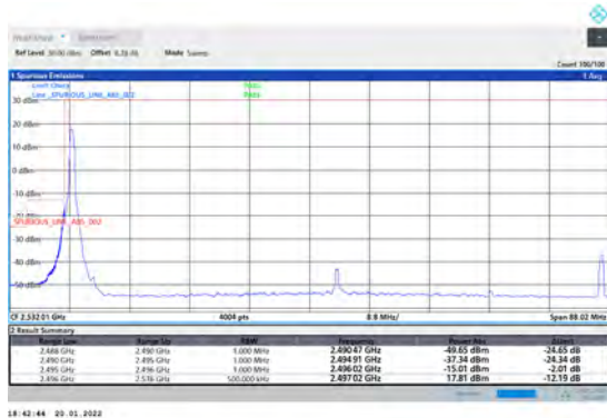
1-N41-PC3-30-80-L-4-CP-QPSK-Edge_1RB_Left-1 @0-Ant1-PASS-see graph
