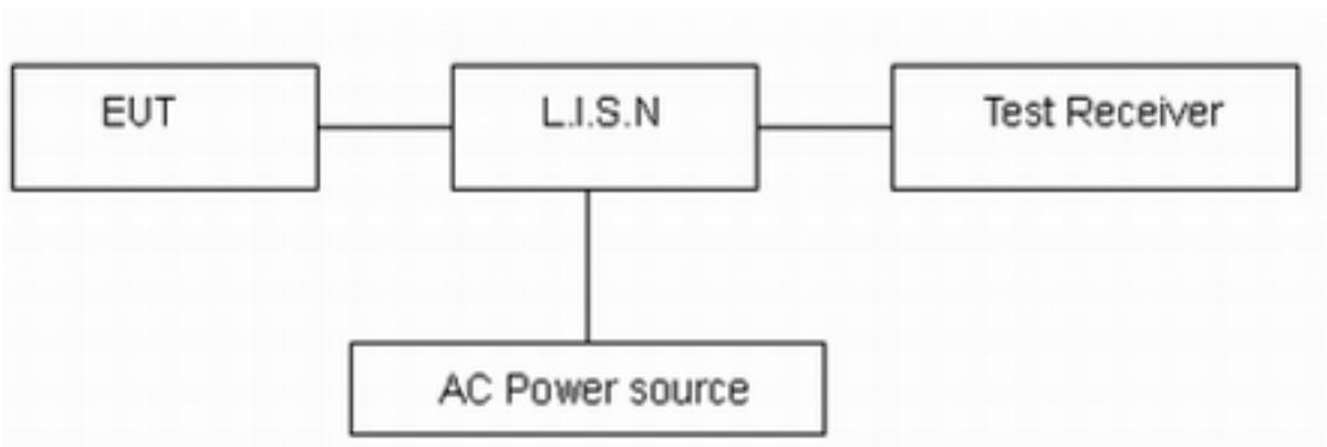
Note: AC Power source is used to change the voltage 110V/60Hz.
