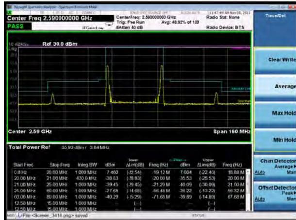
CA\_38C QPSK 20MHz+20MHz CH-High, 1 RB
