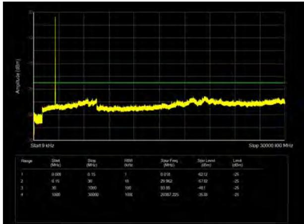
LTE Band 41 20MHz CH-Low 9kHz~30GHz
