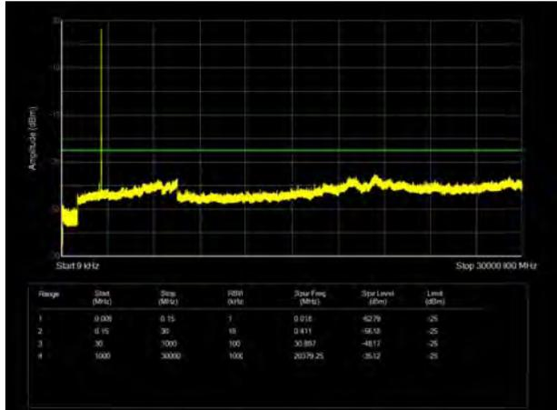
LTE Band 41 10MHz CH- Low 9kHz~30GHz
