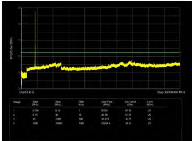
LTE Band 38 20MHz CH-Low 9kHz~30GHz
