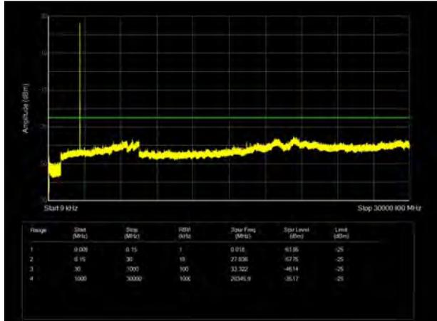
LTE Band 38 10MHz CH- Low 9kHz~30GHz
