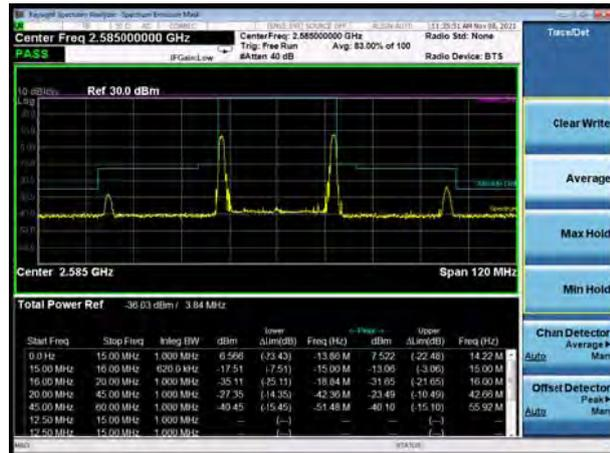
CA\_38C QPSK 15MHz+15MHz CH-High,1 RB
