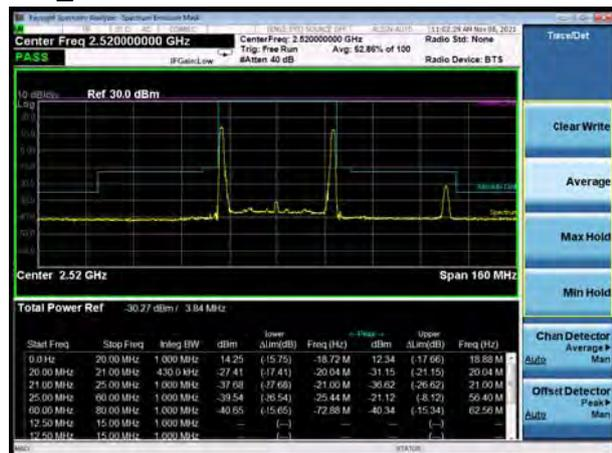
CA\_7C 16QAM 20MHz+20MHz CH-High, 1 RB
