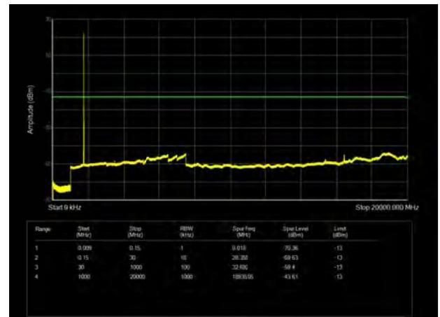
LTE Band 4 5MHz CH-High 9kHz~20GHz
