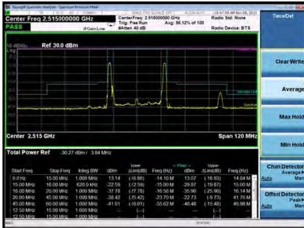
CA\_7C 64QAM 20MHz+10MHz CH-High, 1 RB
