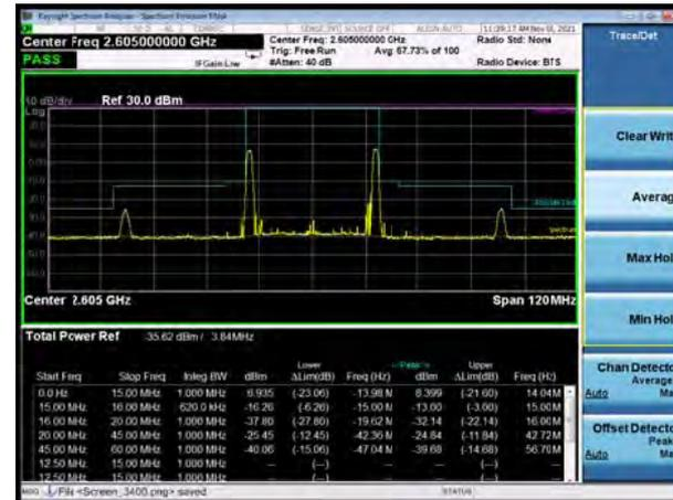
CA\_38C QPSK 15MHz+15MHz CH-Low, 100%RB
