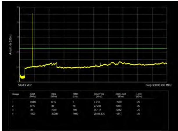
LTE Band 7 20MHz CH-Low 9kHz~30GHz
