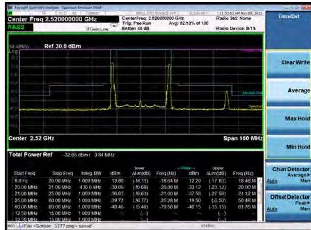
CA\_7C QPSK 20MHz+20MHz CH-High, 1 RB
