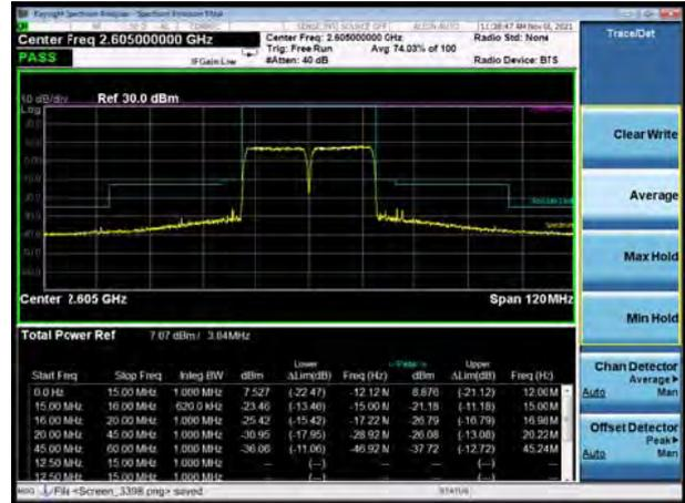
CA\_38C 64QAM 15MHz+15MHz CH-Low,1 RB
