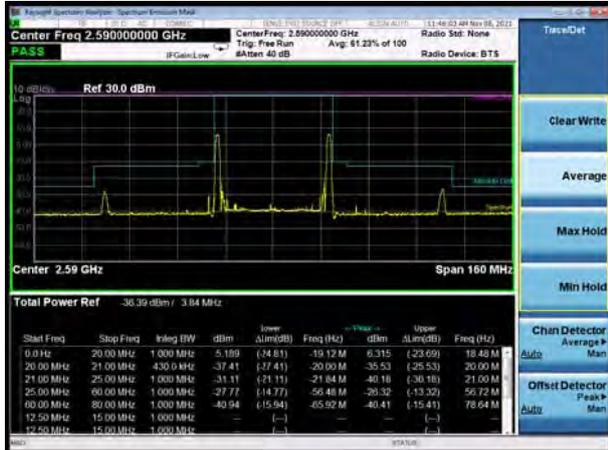
CA\_38C 64QAM 20MHz+20MHz CH-High, 1 RB
