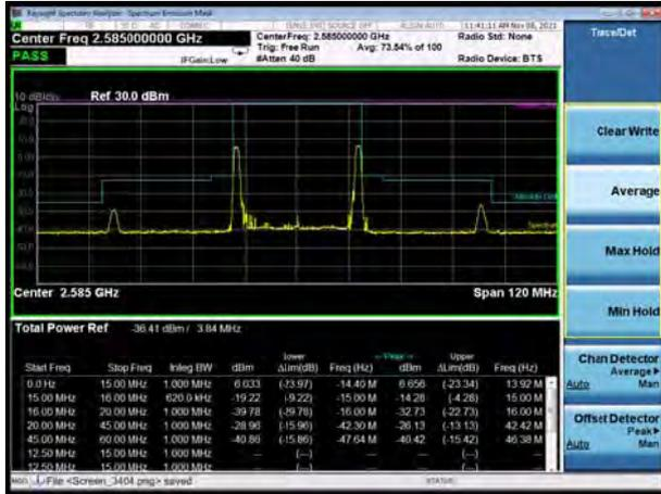
CA\_38C 64QAM 15MHz+15MHz CH-High,1 RB
