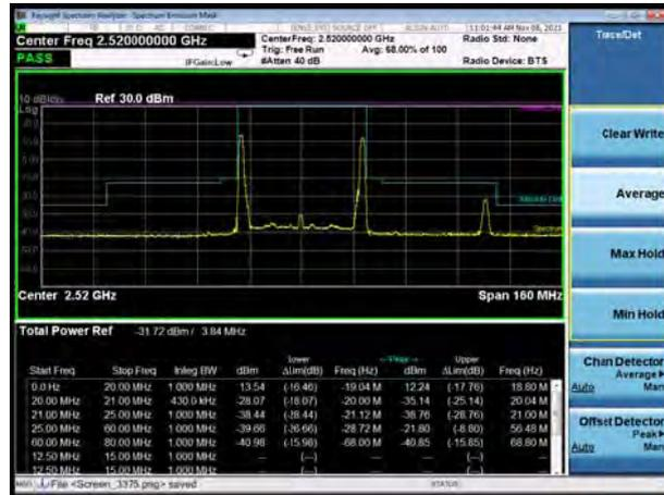
CA\_7C 64QAM 20MHz+20MHz CH-High, 1 RB
