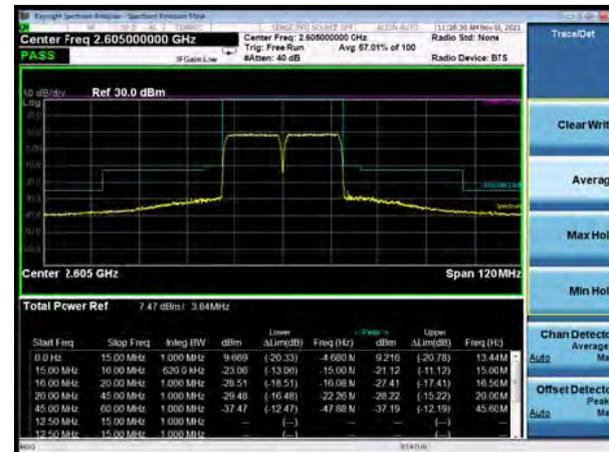
CA\_38C 16QAM 15MHz+15MHz CH-Low,1 RB
