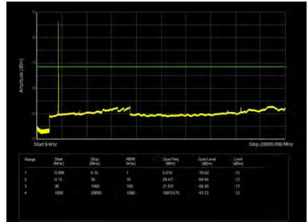
LTE Band 4 5MHz CH- Middle 9kHz~20GHz
