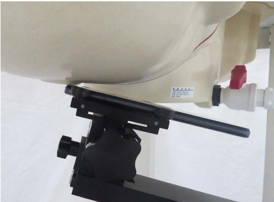
Picture 4: Right Hand Tilt 15 Degree Position
