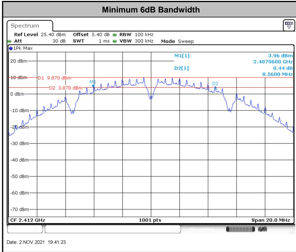
Note : The occupied channel bandwidth is maintained within the band of operation for all of the modulations.
