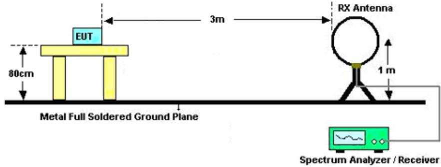
For radiated emissions from 30MHz to 1GHz
