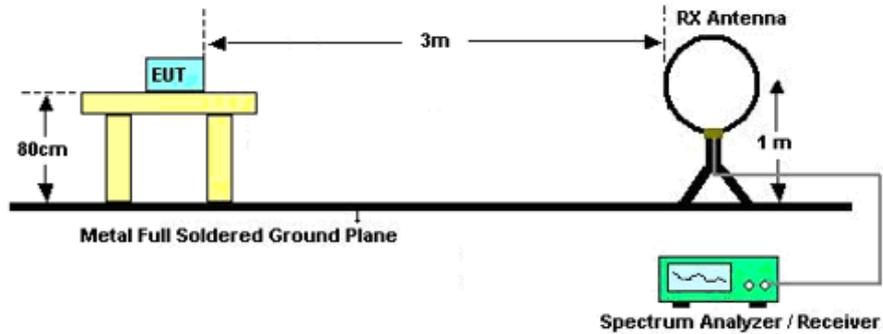
For radiated emissions from 30MHz to 1GHz
