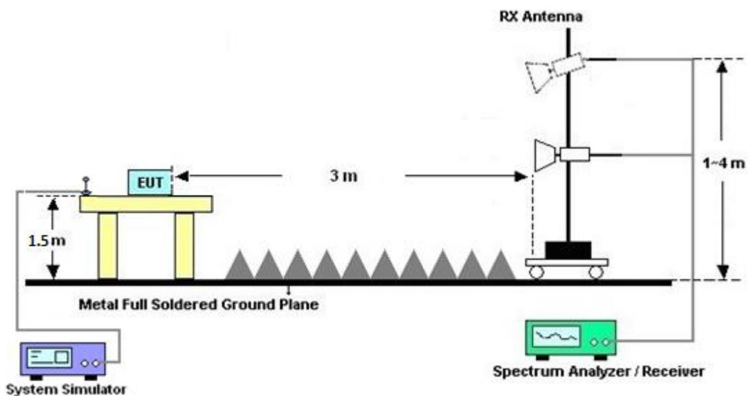
For radiated test above 18GHz
