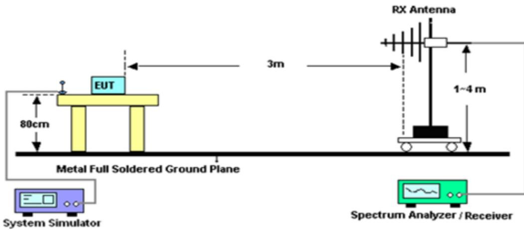
For radiated test from 1GHz to 18GHz
