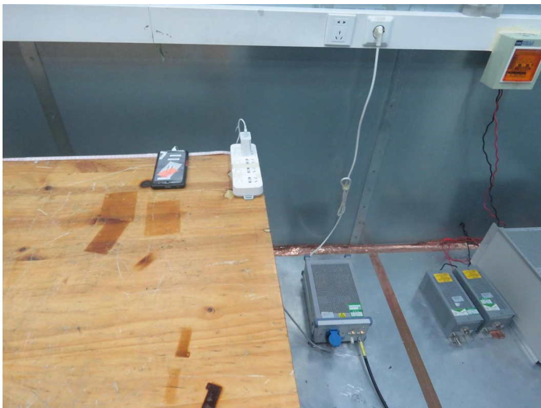
Picture 2 Conducted Emission Test Setup
