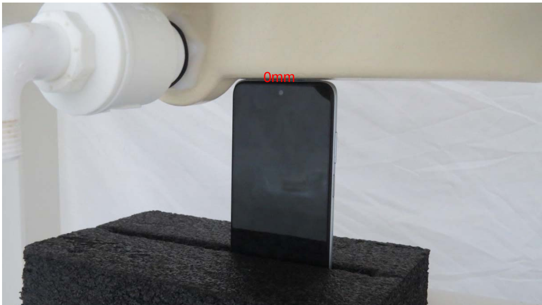
Picture 16: Top Side, the distance from handset to the bottom of the Phantom is 0mm
