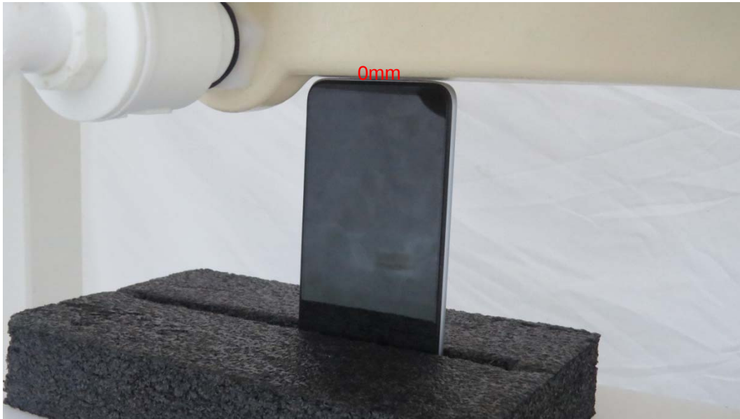
Picture 17: Bottom Edge, the distance from handset to the bottom of the Phantom is 0mm
