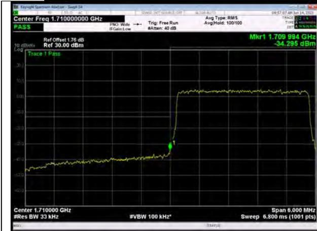
LTE Band 66 16QAM 5MHz CH-Low, 1 RB
