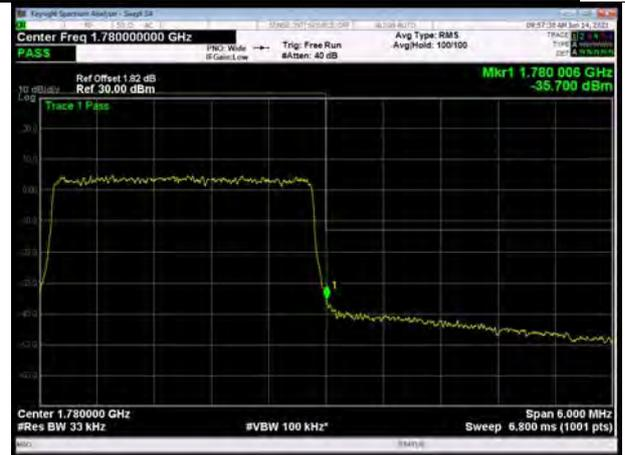
LTE Band 66 16QAM 5MHz CH-High, 1 RB
