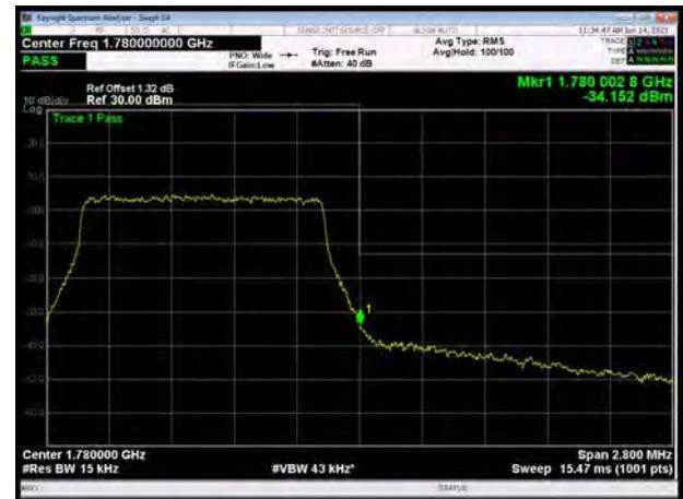
LTE Band 66 64QAM 3MHz CH-Low, 1 RB
