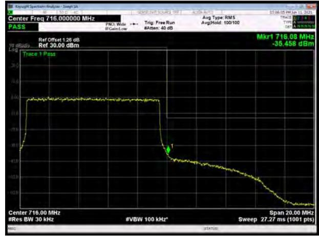
LTE Band 17 16QAM 5MHz CH-Low, 1 RB
