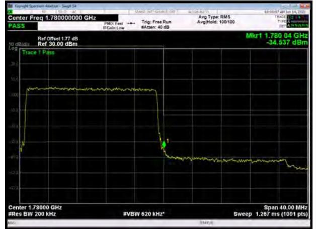
LTE Band 66 16QAM 1.4MHz CH-High, 1 RB
