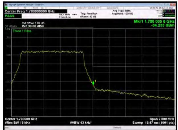
LTE Band 66 16QAM 3MHz CH-Low, 1 RB
