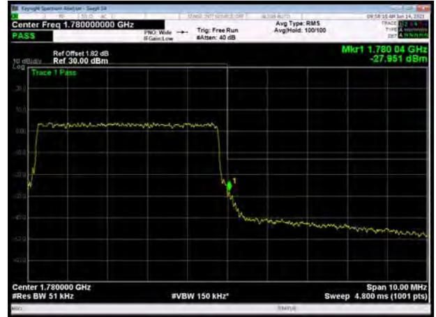
LTE Band 66 16QAM 10MHz CH-High, 1 RB
