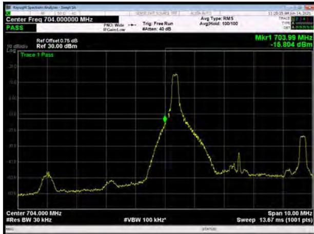
LTE Band 17 64QAM 5MHz CH-High, 1 RB
