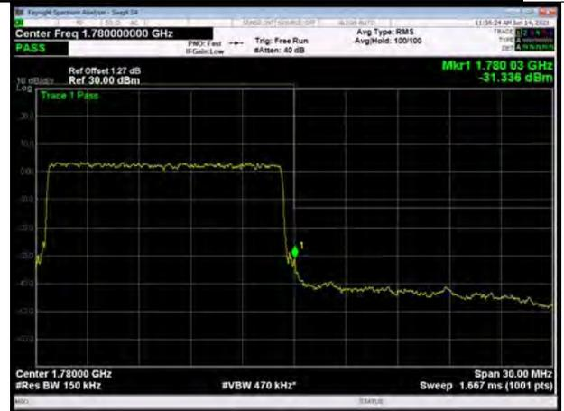
LTE Band 66 64QAM 20MHz CH-High, 1 RB
