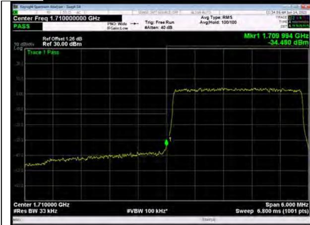
LTE Band 66 64QAM 5MHz CH-Low, 1 RB
