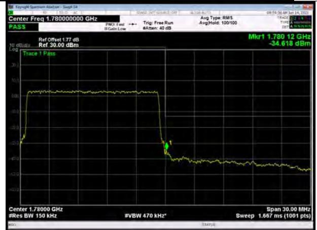
LTE Band 66 16QAM 20MHz CH-High, 1 RB
