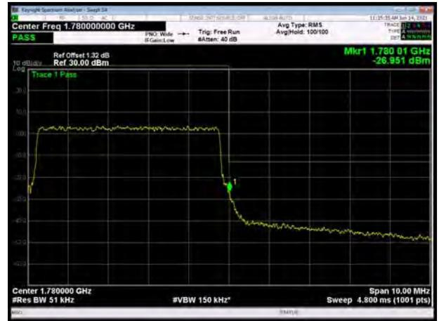
LTE Band 66 64QAM 10MHz CH-High, 1 RB
