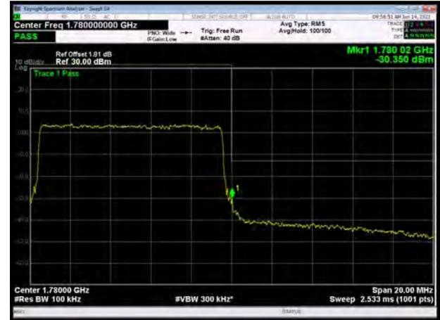
LTE Band 66 16QAM 15MHz CH-Low, 1 RB
