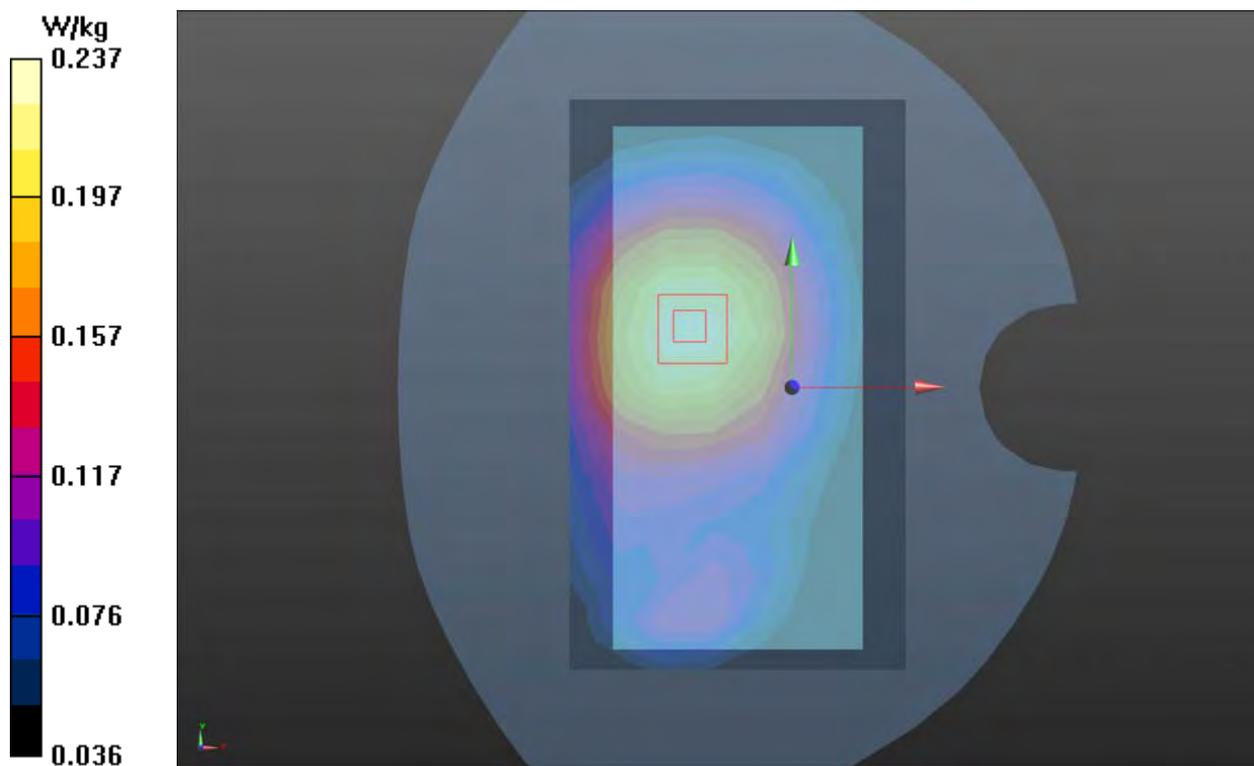
**Plot 38 GSM 1900 Back Side Middle (Distance 15mm)**
