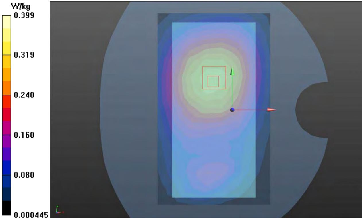
**Plot 63 LTE Band 7 50%RB Front Side High (Distance 10mm)**
