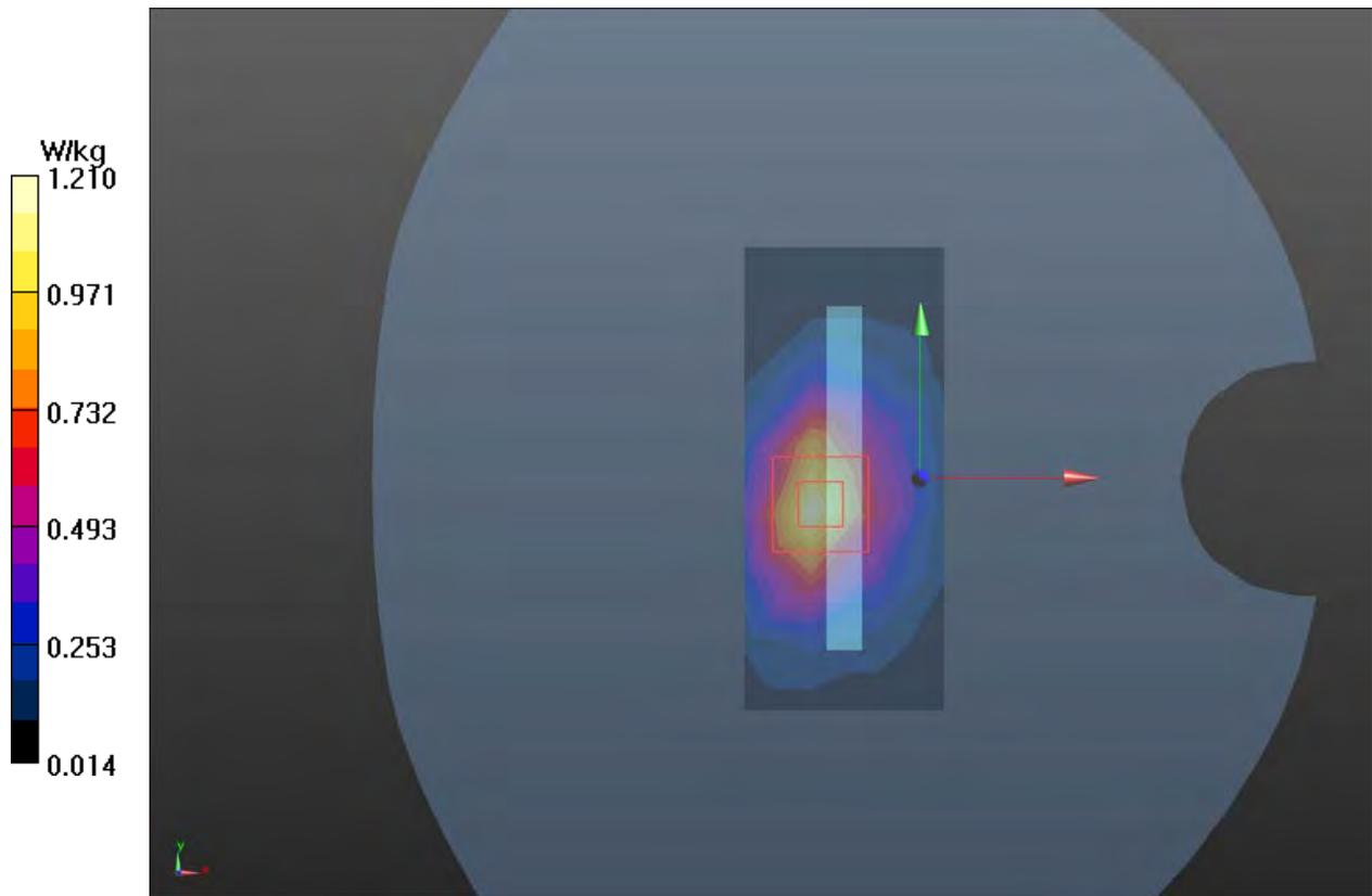
**Plot 57 UMTS Band II Bottom Edge Middle (Distance 10mm)**
