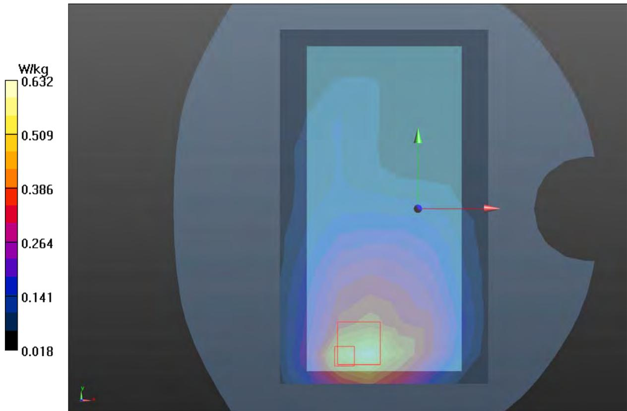
**Plot 44 LTE Band 5 1RB Back Side Low (Distance 15mm)**
