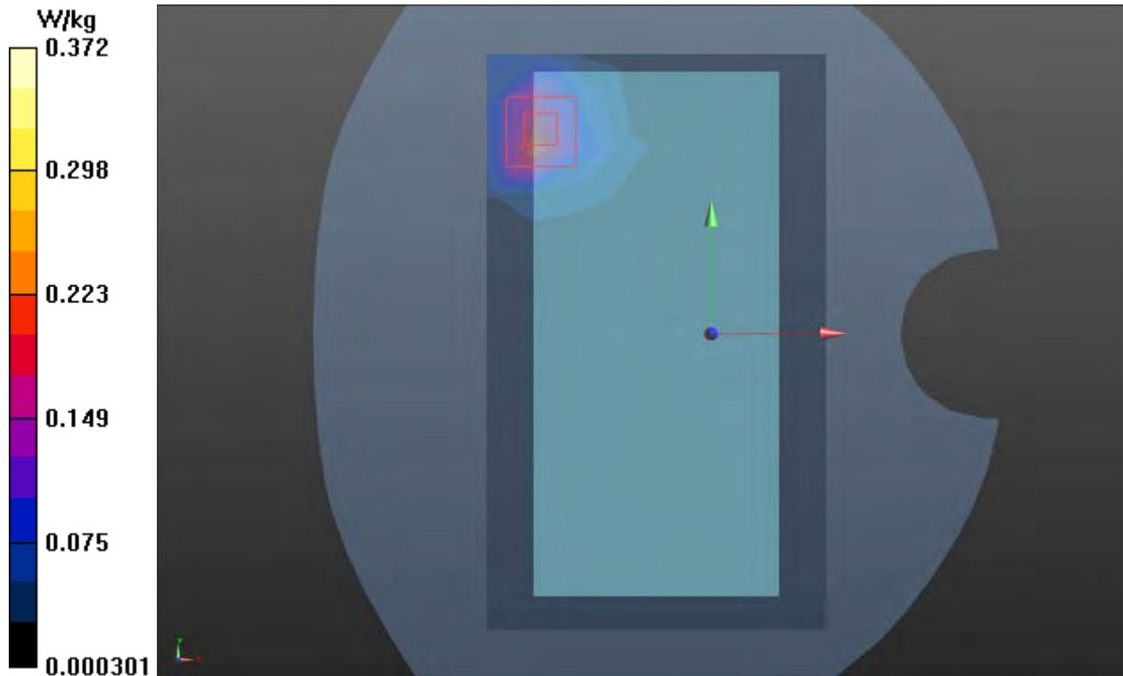
**Plot 55 GSM 850 GPRS (4Txslots) Back Side Middle (Distance 10mm)**
