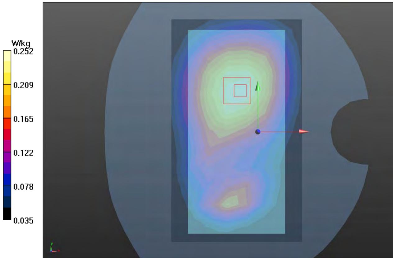
**Plot 42 LTE Band 2 1RB Back Side High (Distance 15mm)**
