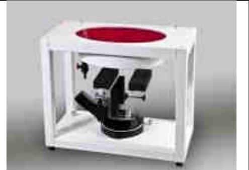
The ELI phantom is intended for compliance testing of handheld and body-mounted wireless devices in the frequency range of 30 MHz to 6 GHz. ELI4 is fully compatible with standard and all known tissue simulating liquids.
