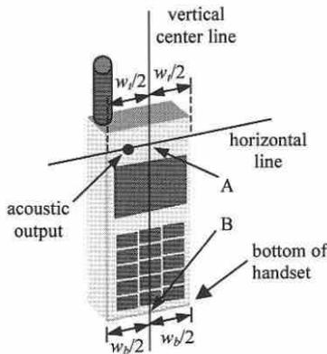
Fig 11.2.1 Handset vertical and horizontal reference lines—“fixed case”
