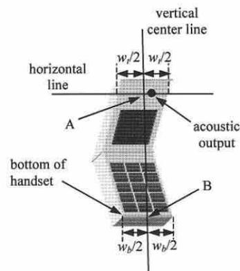
Fig 11.2.2 Handset vertical and horizontal reference lines—“clam-shell case”
