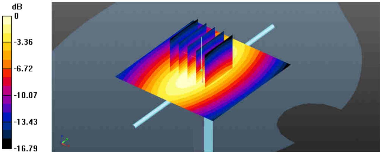
0 dB =  $3.02 \text{ W/kg}$  =  $4.8 \text{ dBW/kg}$
