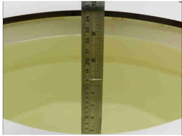
Fig 10.2 Photo of Liquid Height for Body SAR
