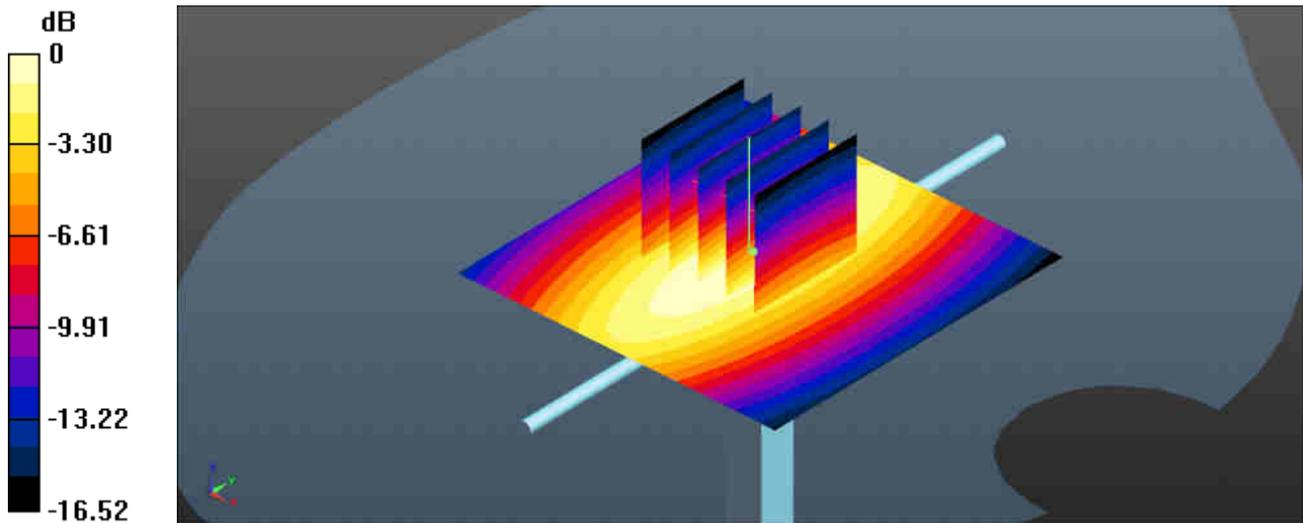
0 dB =  $4.04 \text{ W/kg} = 6.06 \text{ dBW/kg}$
