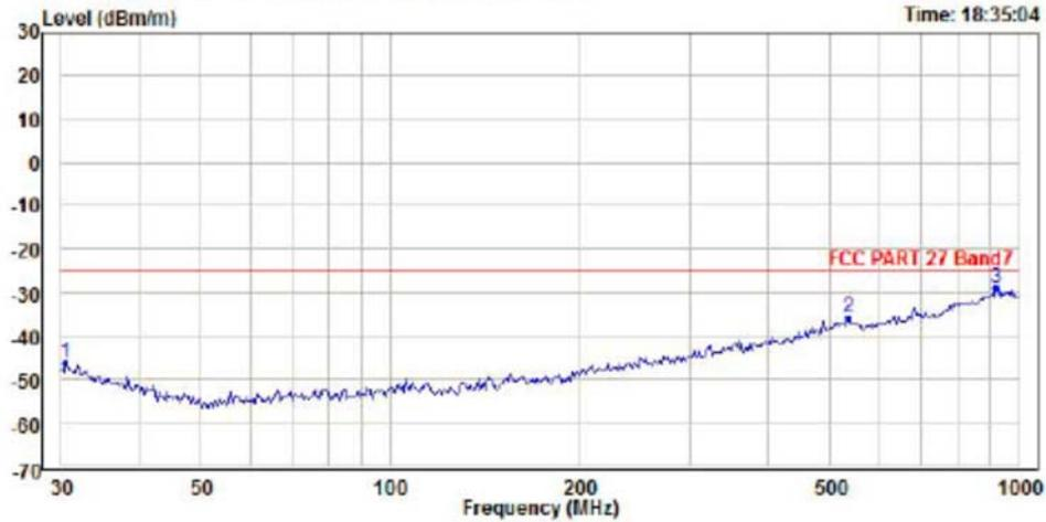
Condition : limit\FCC\FCC PART 27 Band7.csv 3m Vertical
