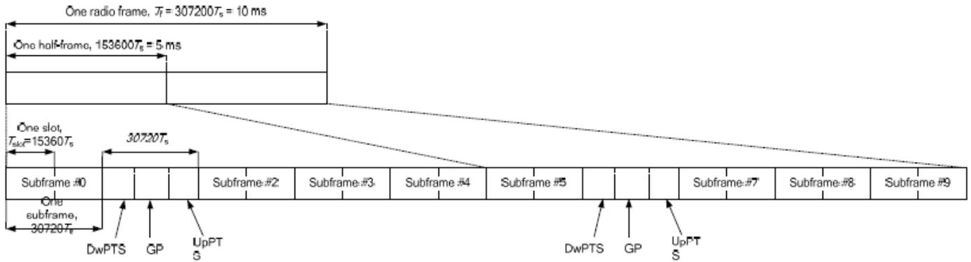
**Figure 4.2-1: Frame structure type 2 (for 5 ms switch-point periodicity).**
