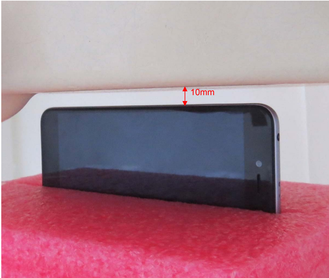
Picture 20: Left Side, the distance from handset to the bottom of the Phantom is 10mm
