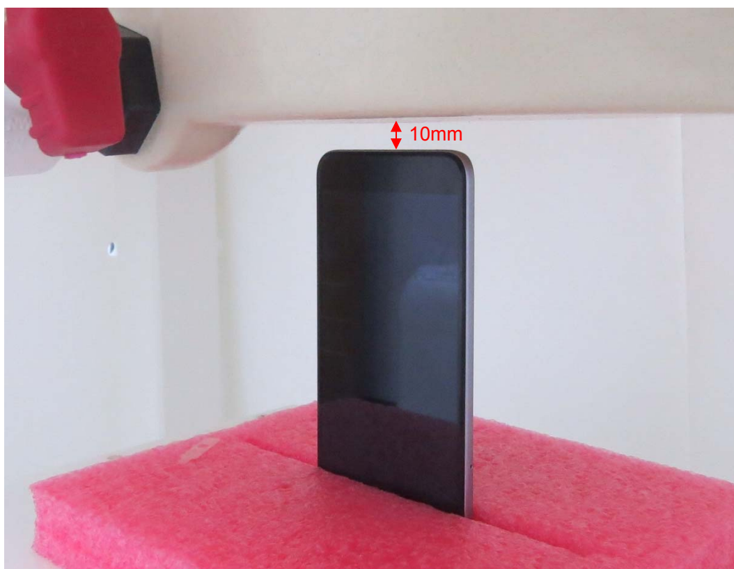
Picture 23: Bottom Side, the distance from handset to the bottom of the Phantom is 10mm
