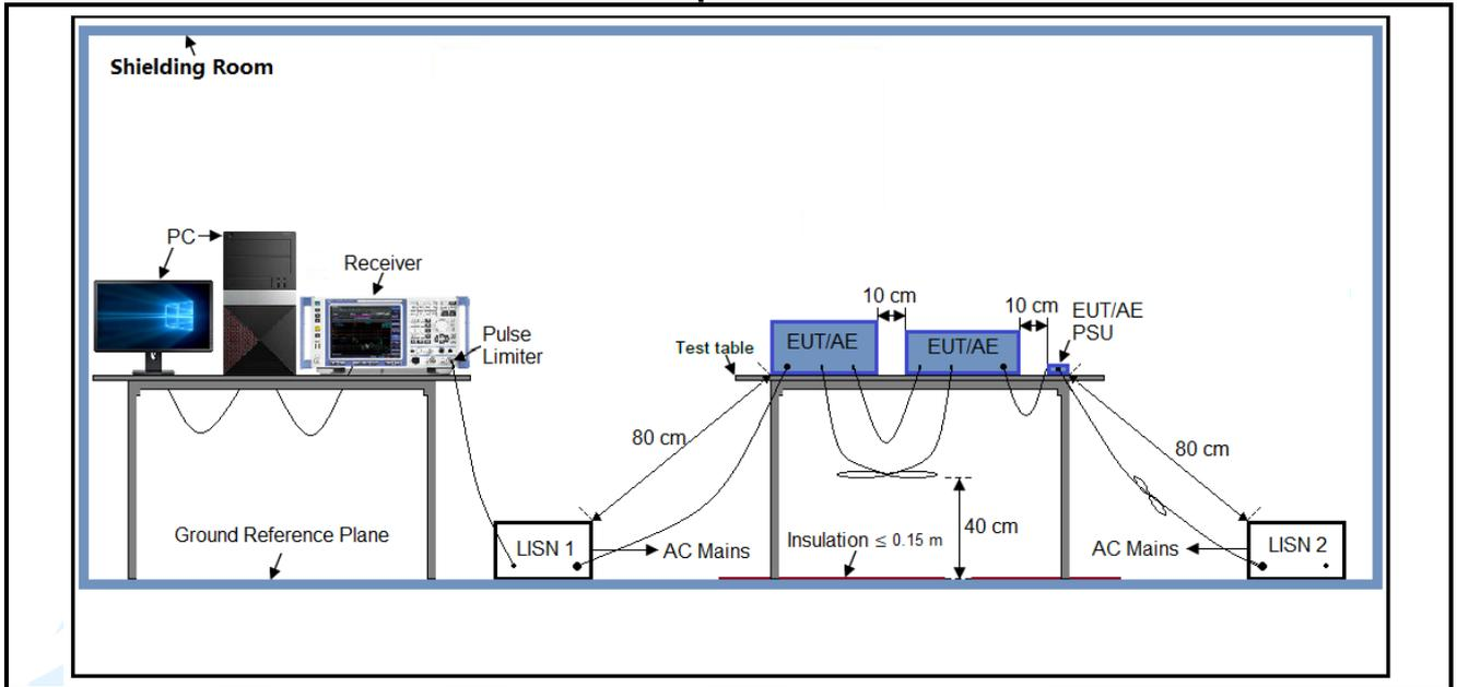
4.4.3 For Conducted RF test setup
