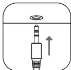
Plug the 3.5 mm AUX cable into your car's AUX port. Turn your car stereo to the AUX mode.
