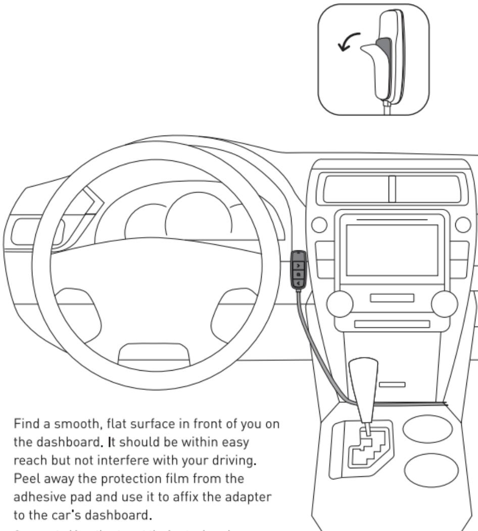
Find a smooth, flat surface in front of you on the dashboard. It should be within easy reach but not interfere with your driving. Peel away the protection film from the adhesive pad and use it to affix the adapter to the car's dashboard.
