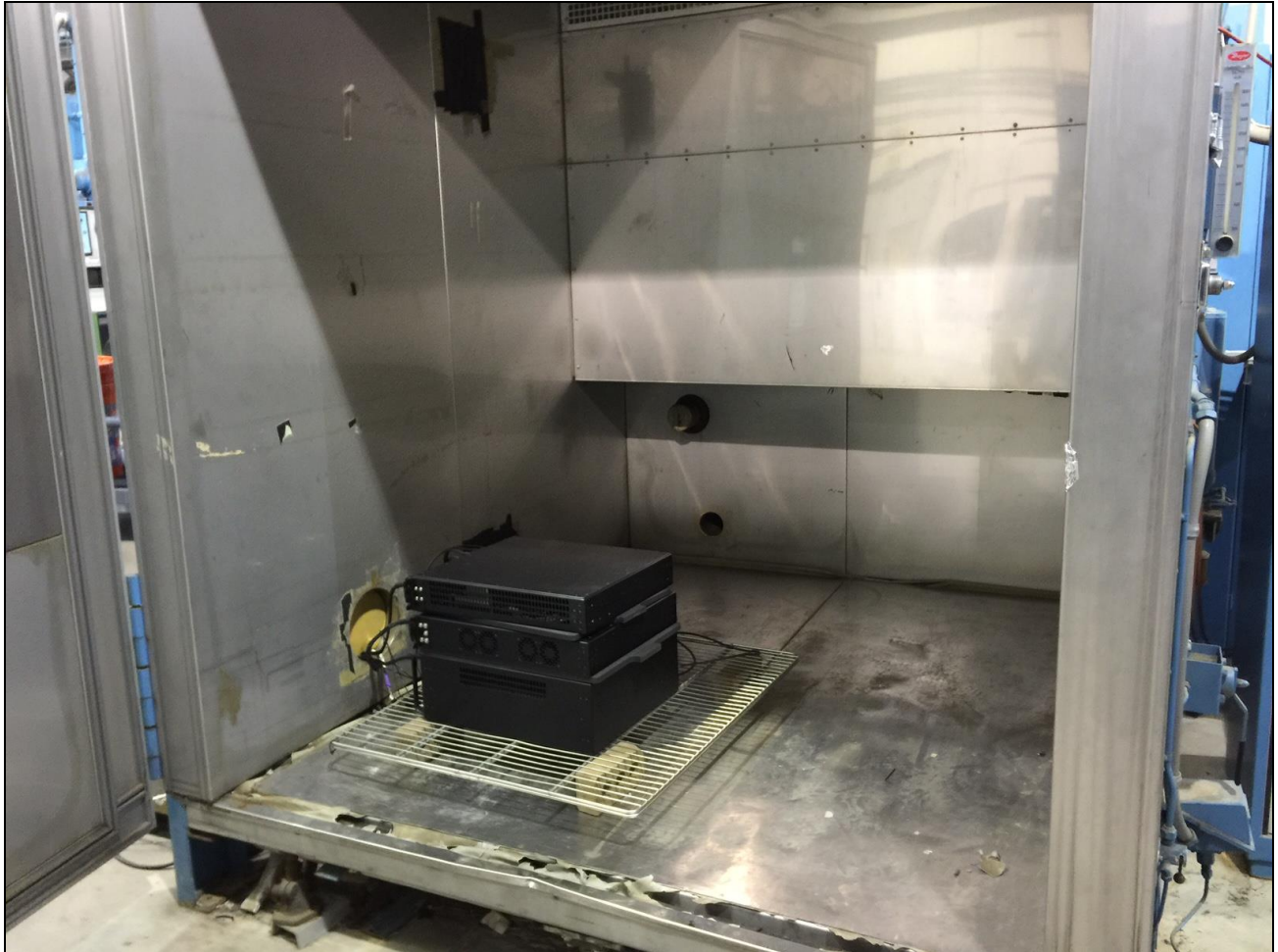
Photograph 2. Frequency Stability, Test Setup
