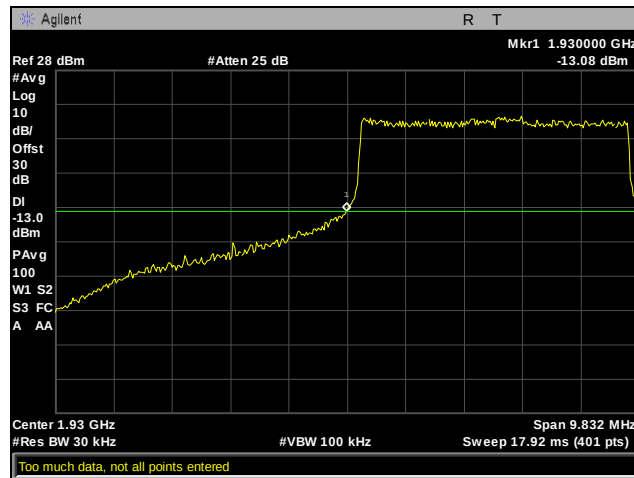
Plot 248. Conducted Band Edge, Channel 625, 5 MHz, Part 24
