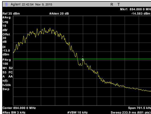
Plot 57. Conducted Band Edge, Channel 251, Part 22
