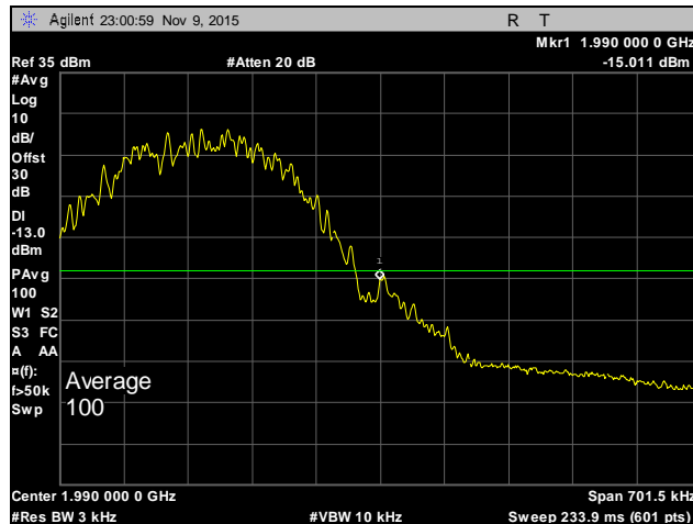
Plot 59. Conducted Band Edge, Channel 810, Part 24
