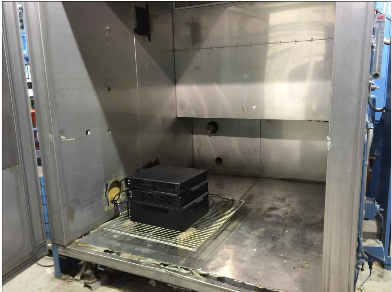
Photograph 2. Frequency Stability, Test Setup
