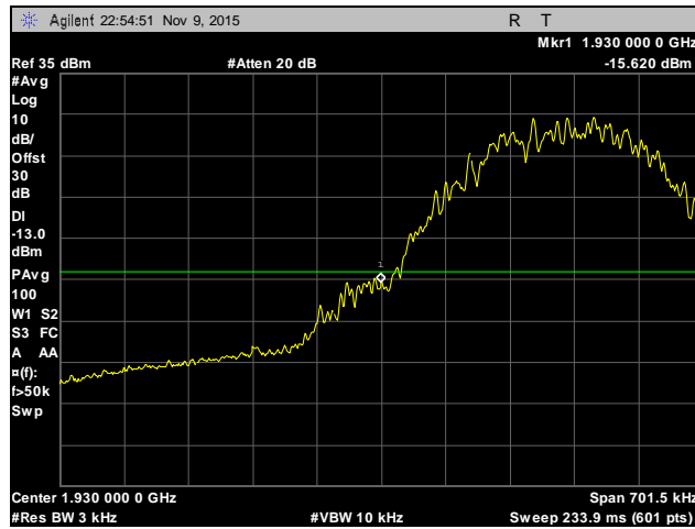
Plot 58. Conducted Band Edge, Channel 512, Part 24
