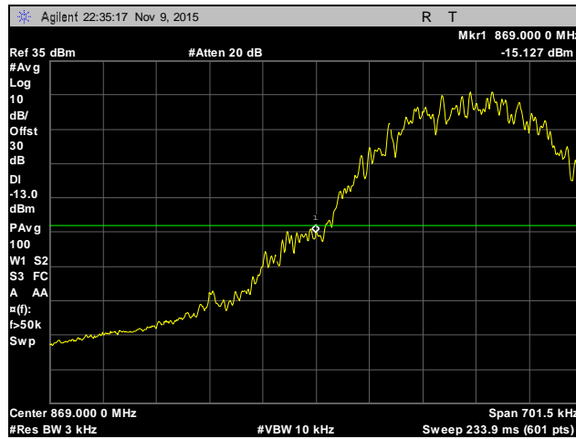
Plot 56. Conducted Band Edge, Channel 128, Part 22
