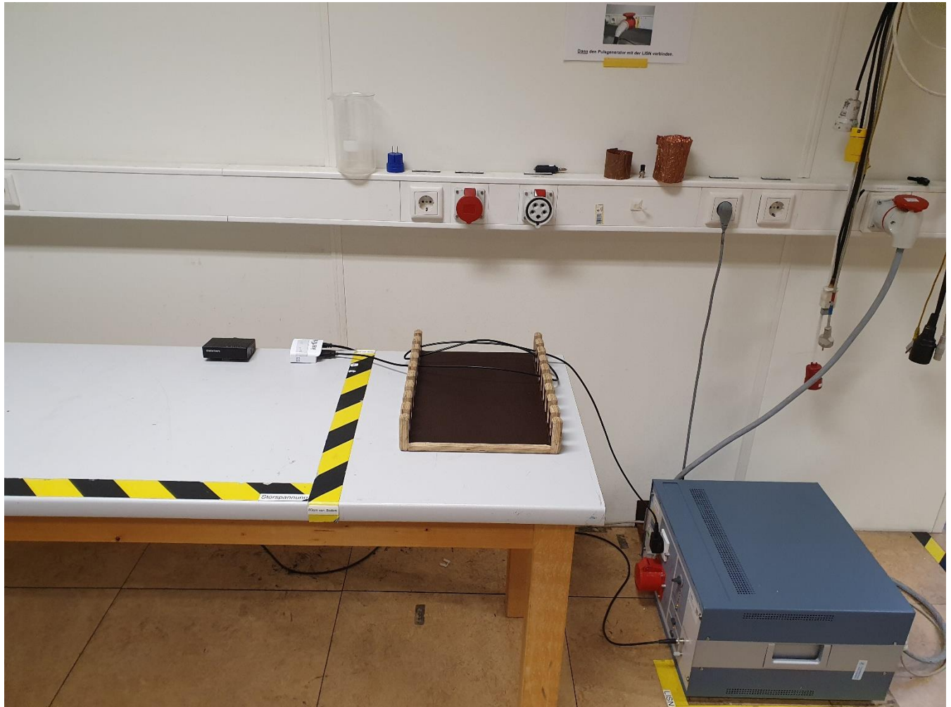
Bild / Picture 3: Test Setup, Radiated disturbance (> 1 GHz)
