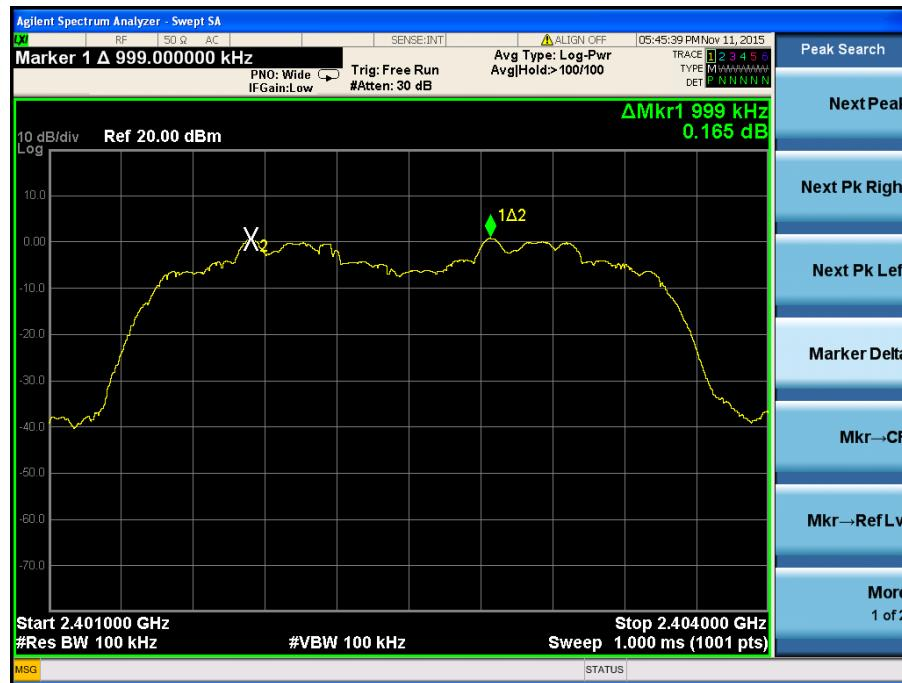
Channel Spacing (Middle CH=1MHz)
