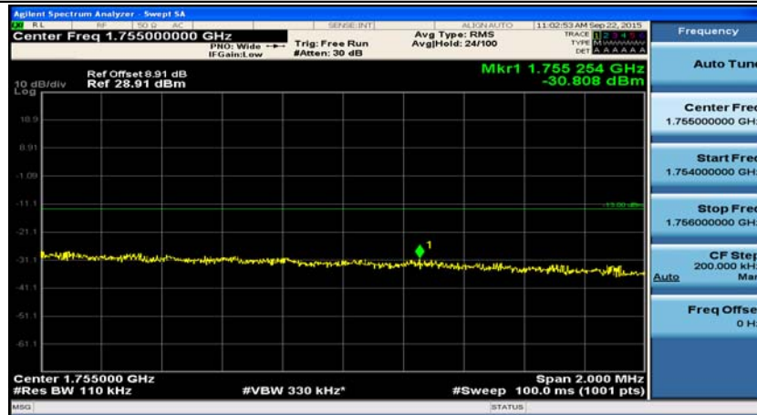
Channel Bandwidth: 10 MHz_HCH_16QAM_25RB#25
