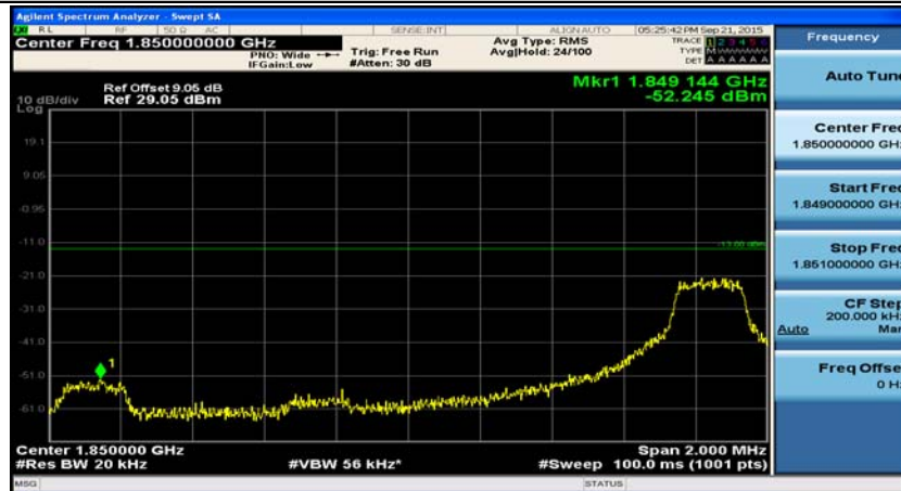
(Channel Bandwidth:15 MHz)_LCH_16QAM_37RB#0
