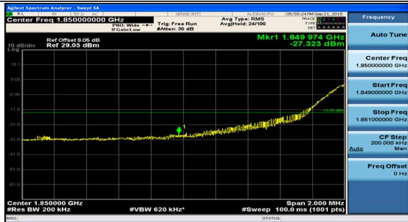
(Channel Bandwidth:20 MHz)_LCH_QPSK_50RB#25
