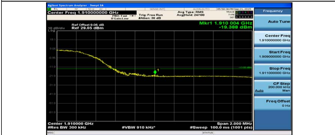
(Channel Bandwidth:15 MHz)_HCH_QPSK_75RB#0
