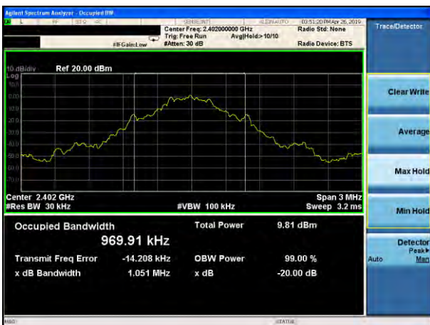
20dB Bandwidth plot on channel 39 (1Mbps)
