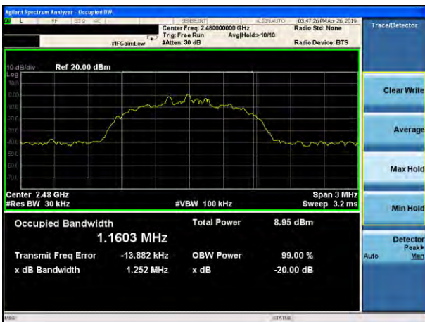
20dB Bandwidth plot on channel 78 (3Mbps)
