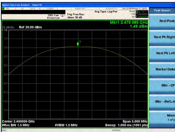
Peak output Power plot on channel 78 (1Mbps)
