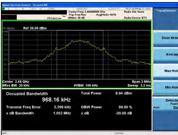
20dB Bandwidth plot on channel 78 (1Mbps)
