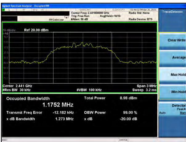
20dB Bandwidth plot on channel 39 (3Mbps)
