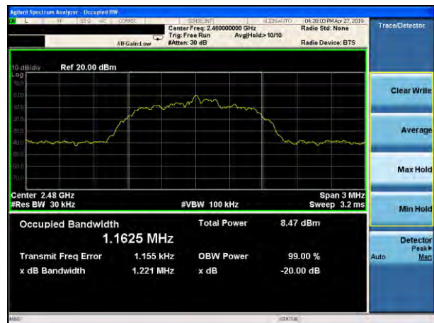
20dB Bandwidth plot on channel 78 (2Mbps)
