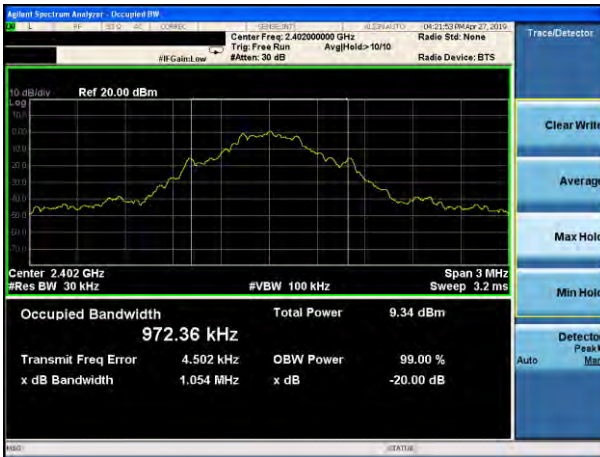
20dB Bandwidth plot on channel 39 (1Mbps)
