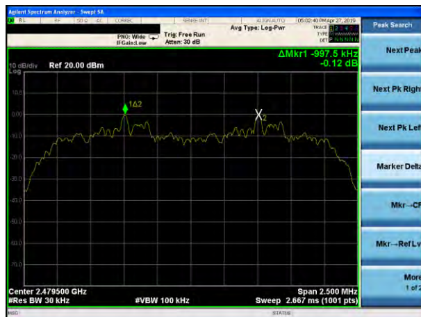
(2Mbps) Channel Separation plot on channel 77-78
