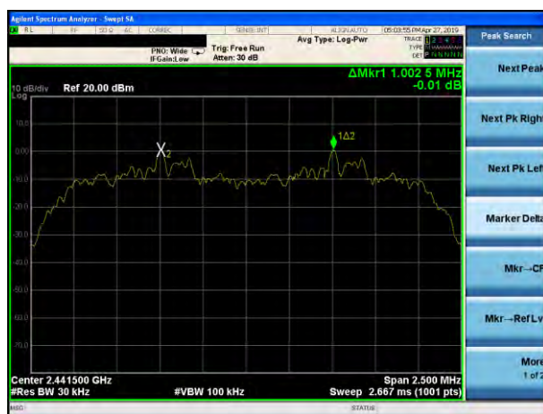
(2Mbps) Channel Separation plot on channel 39-40
