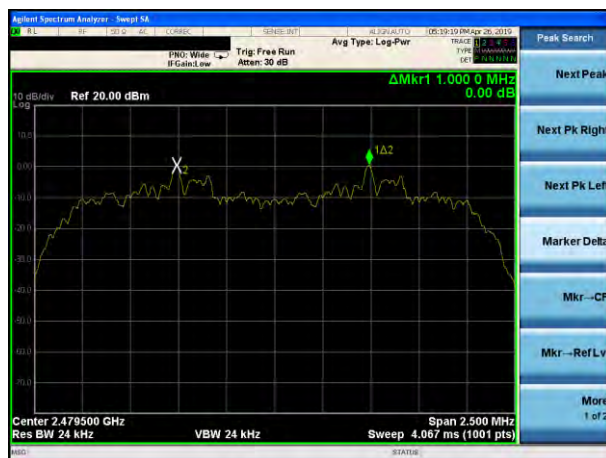
(2Mbps) Channel Separation plot on channel 77-78
