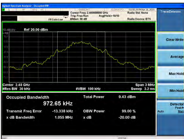
20dB Bandwidth plot on channel 78 (1Mbps)
