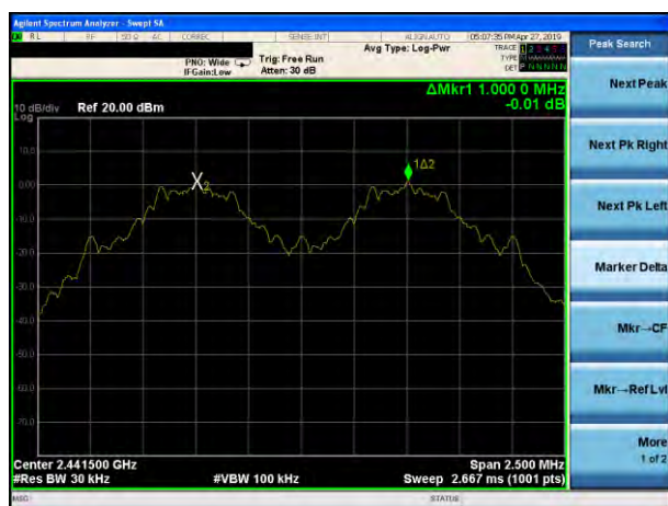
(1Mbps) Channel Separation plot on channel 39-40
