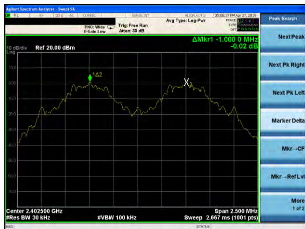
(1Mbps) Channel Separation plot on channel 00-01
