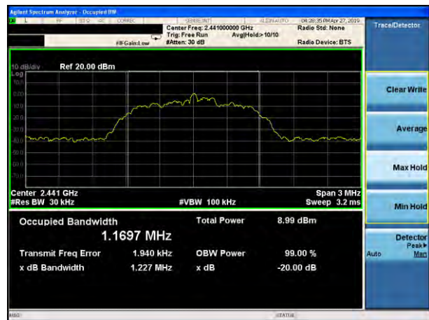
20dB Bandwidth plot on channel 78 (2Mbps)
