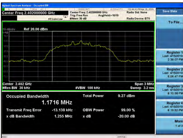
20dB Bandwidth plot on channel 00 (3Mbps)
