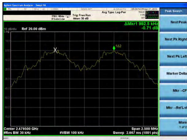
(1Mbps) Channel Separation plot on channel 77-78
