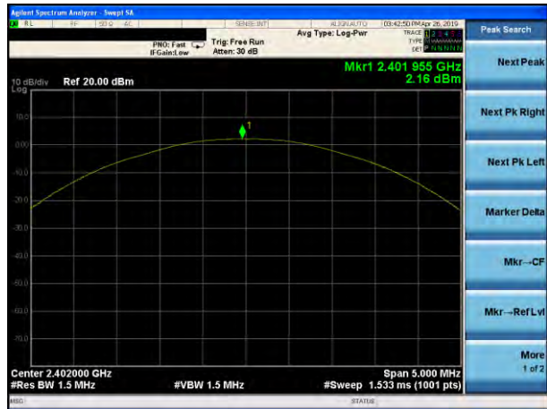
Peak output Power plot on channel 00 (2Mbps)
