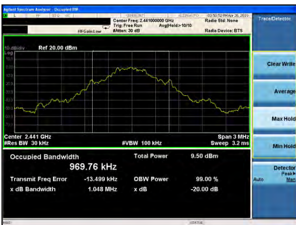
20dB Bandwidth plot on channel 78 (1Mbps)
