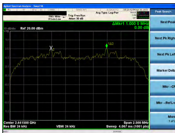
(2Mbps) Channel Separation plot on channel 39-40
