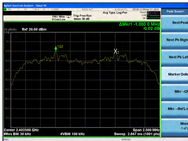
(2Mbps) Channel Separation plot on channel 00-01
