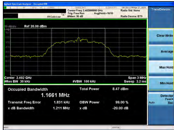
20dB Bandwidth plot on channel 39 (2Mbps)
