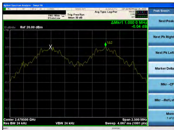
(1Mbps) Channel Separation plot on channel 77-78
