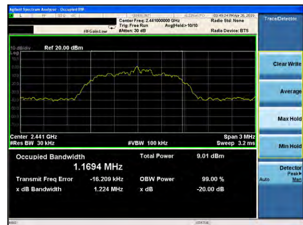
20dB Bandwidth plot on channel 78 (2Mbps)
