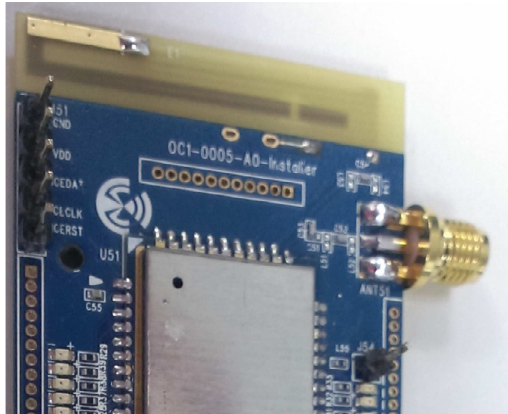
Figure15-1.Reversed SMA connector to connect dipole antenna
