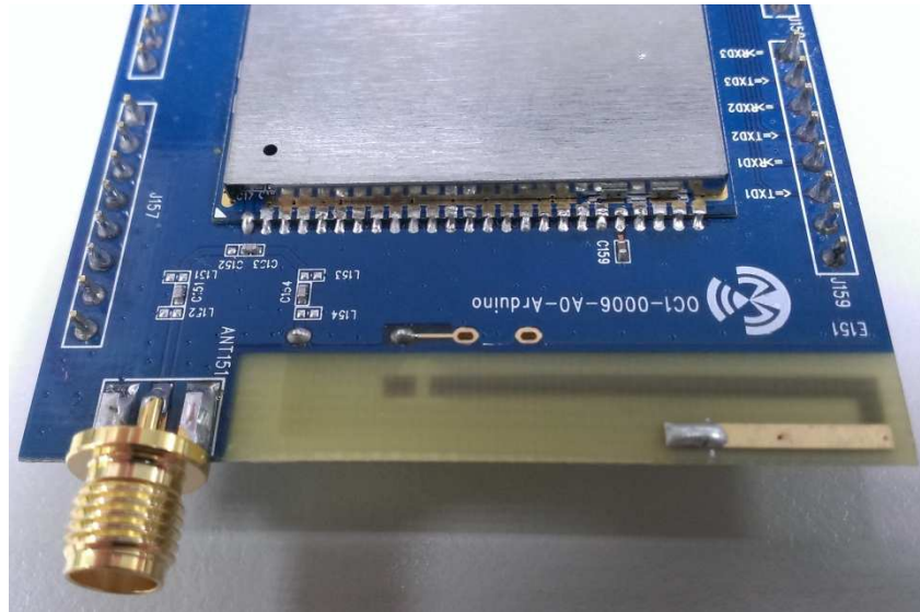
Figure11-1.Reversed SMA connector to connect dipole antenna
