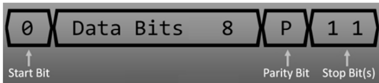
Figure7. UART Data Format
