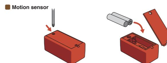
Use a cross slot screwdriver to loosen the screw on the reverse side of the motion sensor and insert the provided AAA batteries. The sensor will boot up automatically. The AAA batteries are provided for first-time setup; replacement batteries may be required for prolonged use.
