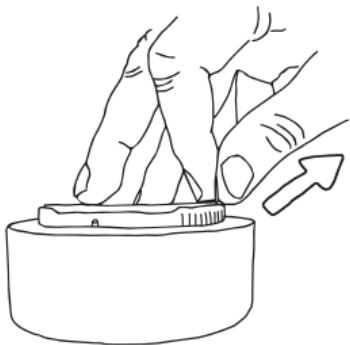
Remove the mounting plate from Point by pulling the tab.
