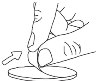
Install the mounting plate on the ceiling. Use the provided sticky tape or a screw.
