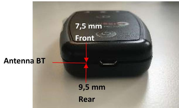
Accordingly with the Bluegiga report we can confirm that the Bluetooth transmission operates in the BT121 module for 300,1ms in a period of 31,6 seconds, we can treat the object of the par.6.3 of the KDB 447489 D01 "General RF Exposure Guidance" v06 and considering the HC1000 as Low transmission duty factor device.
