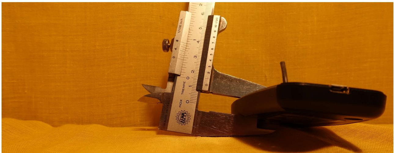
We taking into account that **the housing grantee a minimum distance of 7.5 mm** as separation between the Bluetooth antenna inside the device and the closest hand surface in contact with the external device in the correlated point of the Bluetooth antenna. Accordingly with this our measurements and the SILICON Lab evaluation about the SAR, we can confirm on the HC1000 that the SAR measurement can be excluded.
