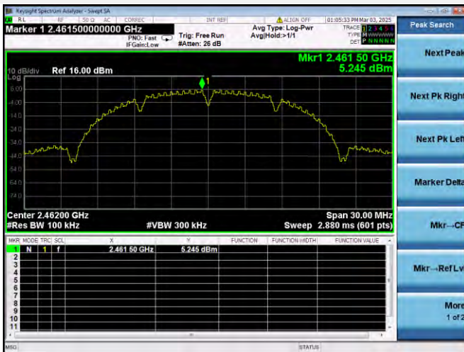
802.11b HIGH CHANNEL, CARRIER LEVEL
