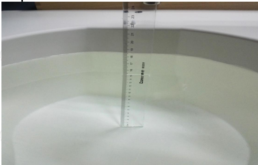
The Body Liquid of 2450MHz (15.3cm)
