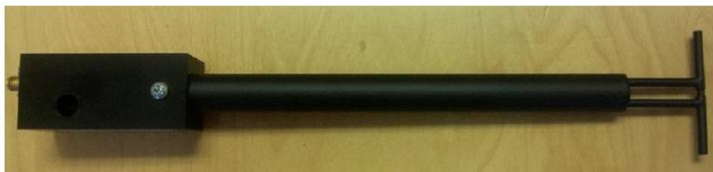
Figure 1 – MVG COMOSAR Validation Dipole
