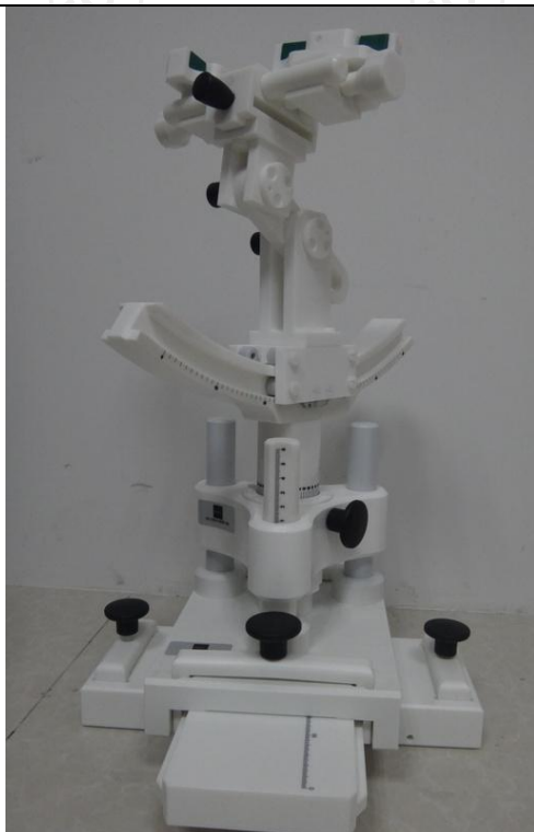
COMOSAR Mobile phone positioning system
