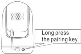
The camera can be connected both to the monitor and the App. Generally, it is connected to the monitor by default. Follow the steps below to connect the camera to the App.
