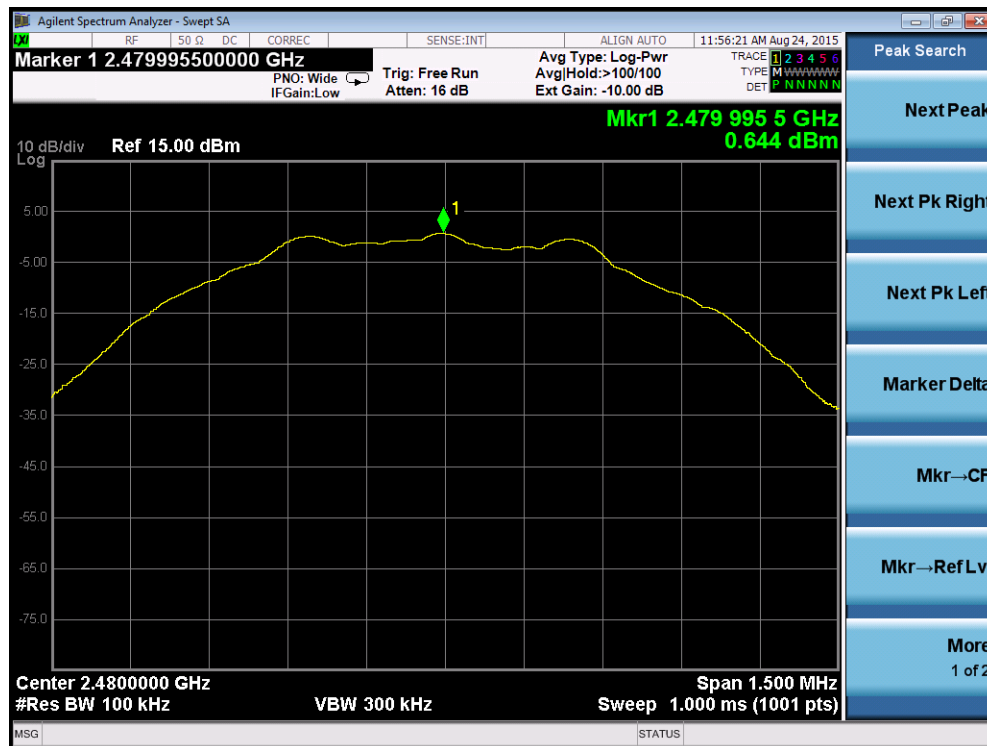
High Channel – Peak Power Spectral Density
