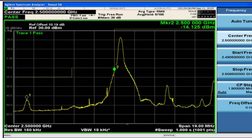
Channel Bandwidth: 10 MHz_LCH_16QAM_1RB#24
