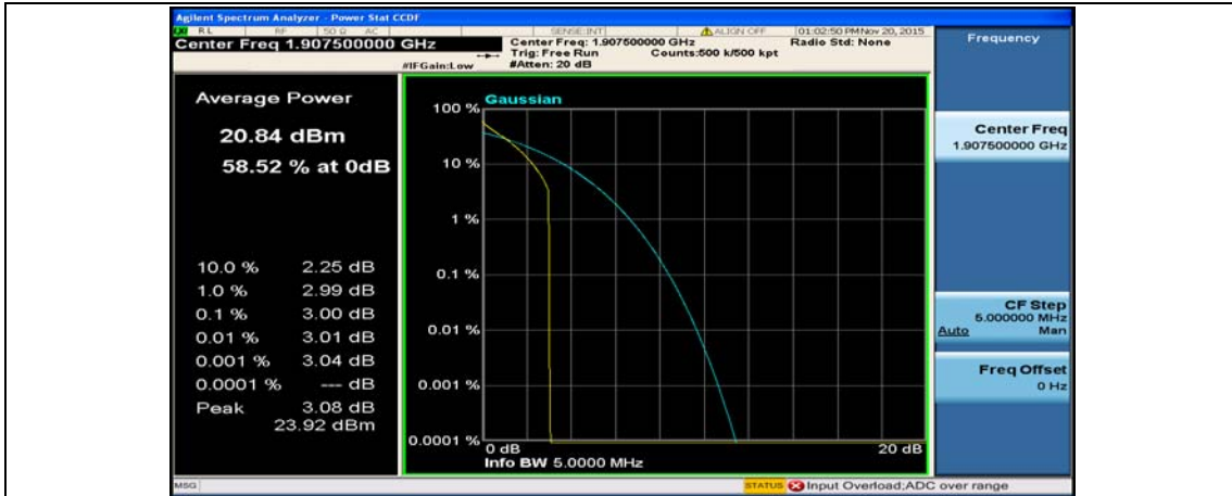
(Channel Bandwidth: 5 MHz)_HCH_16QAM_1RB#24
