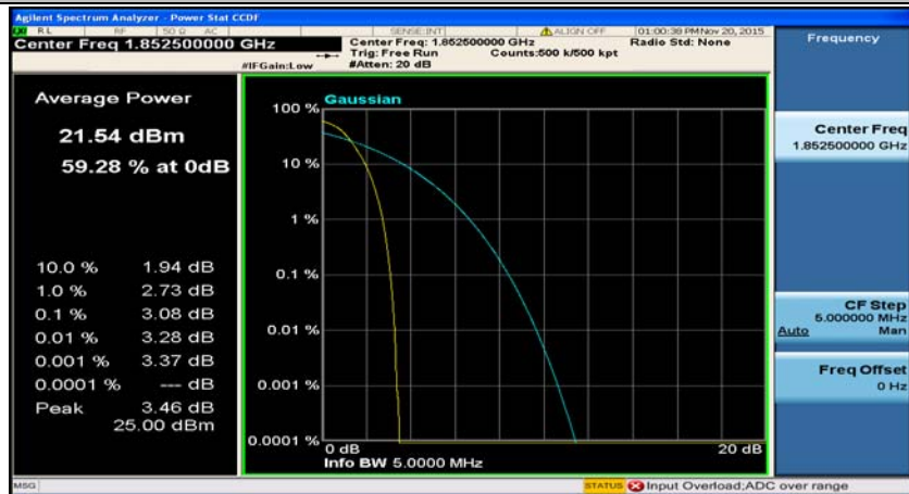
(Channel Bandwidth: 5 MHz)_LCH_16QAM_25RB#0
