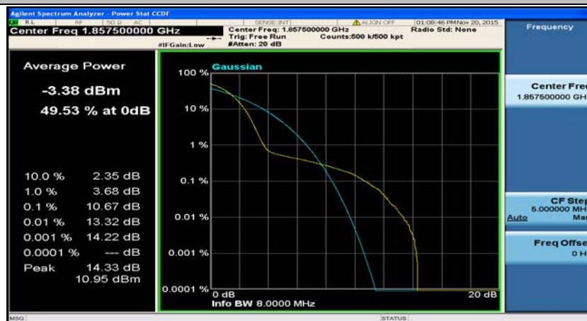
(Channel Bandwidth:15 MHz)_LCH_16QAM_37RB#0
