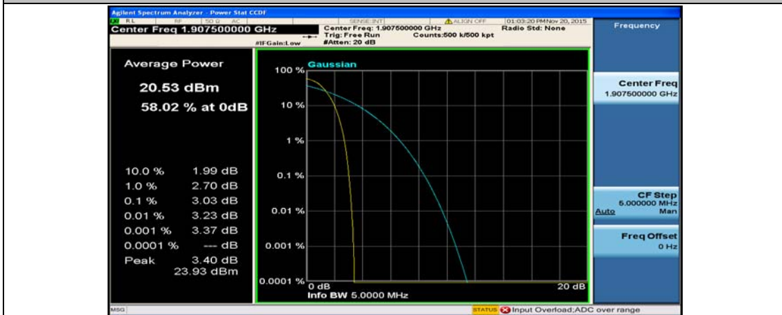
(Channel Bandwidth: 5 MHz)_HCH_16QAM_12RB#6
