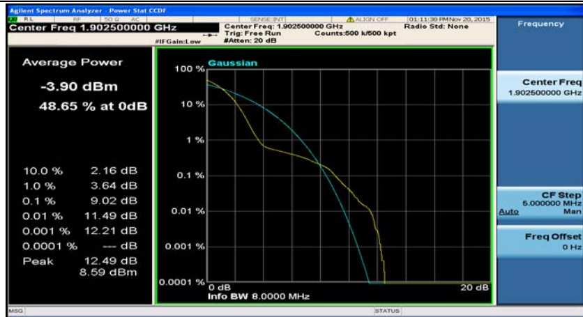
(Channel Bandwidth:15 MHz)_HCH_QPSK_37RB#0
