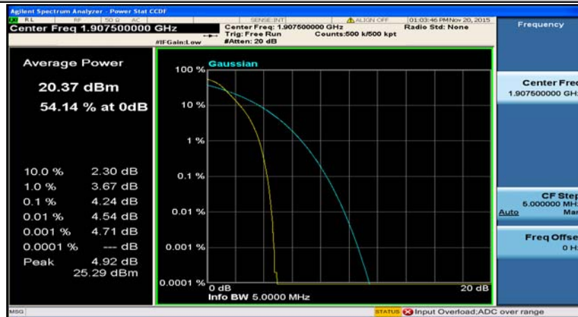
(Channel Bandwidth: 5 MHz)_HCH_16QAM_25RB#0
