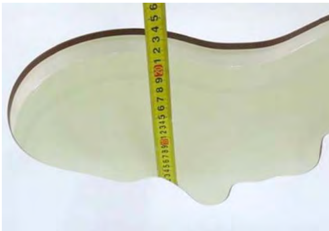
Picture 19: Liquid depth in the head Phantom (5800 MHz, 15.1cm depth)
