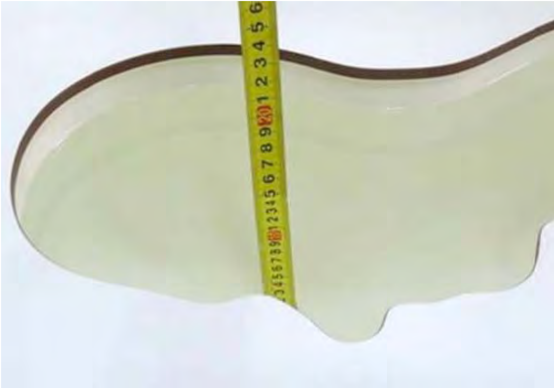
Picture 15: Liquid depth in the head Phantom (5300 MHz, 15.4cm depth)
