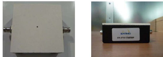
Figure 1 – MVG COMOHAC Magnetic Field Simulator
