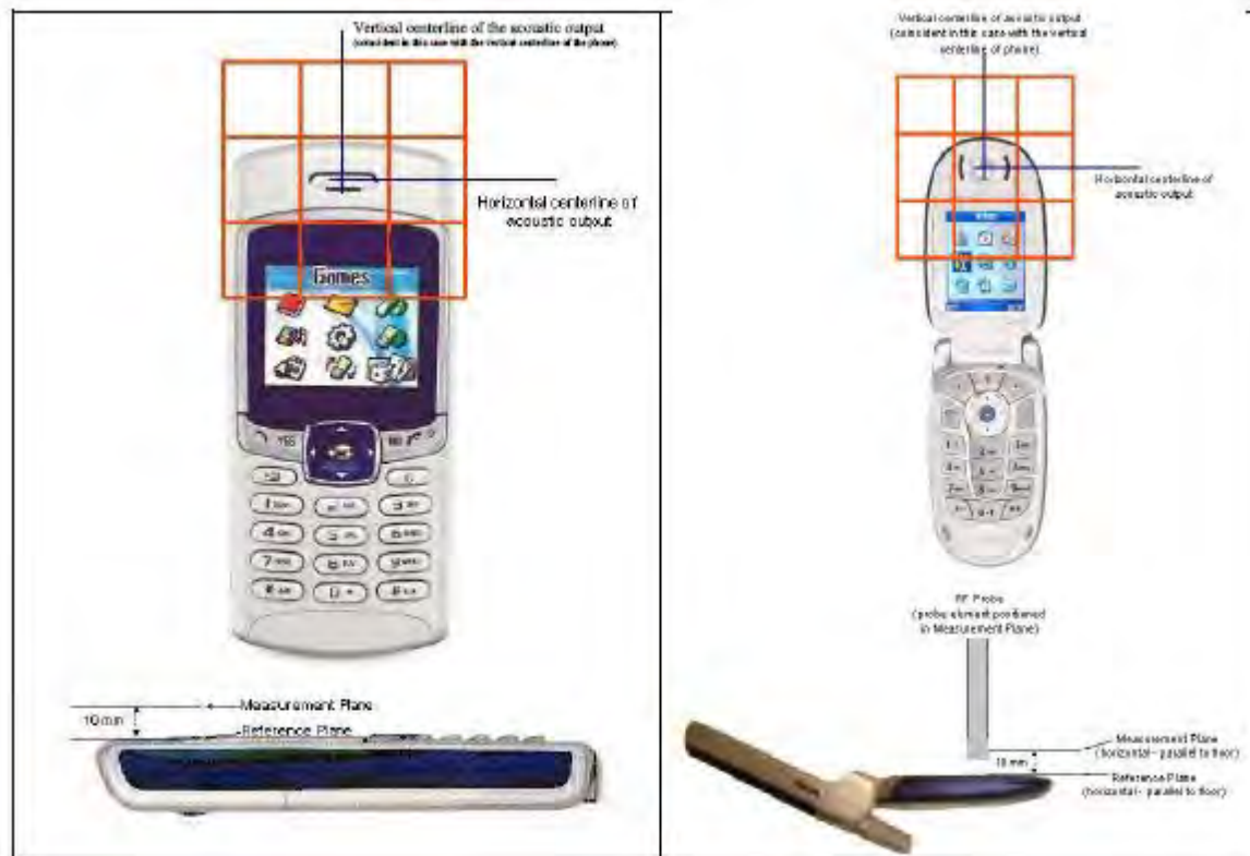
Reference and plane for RF emission measurements
