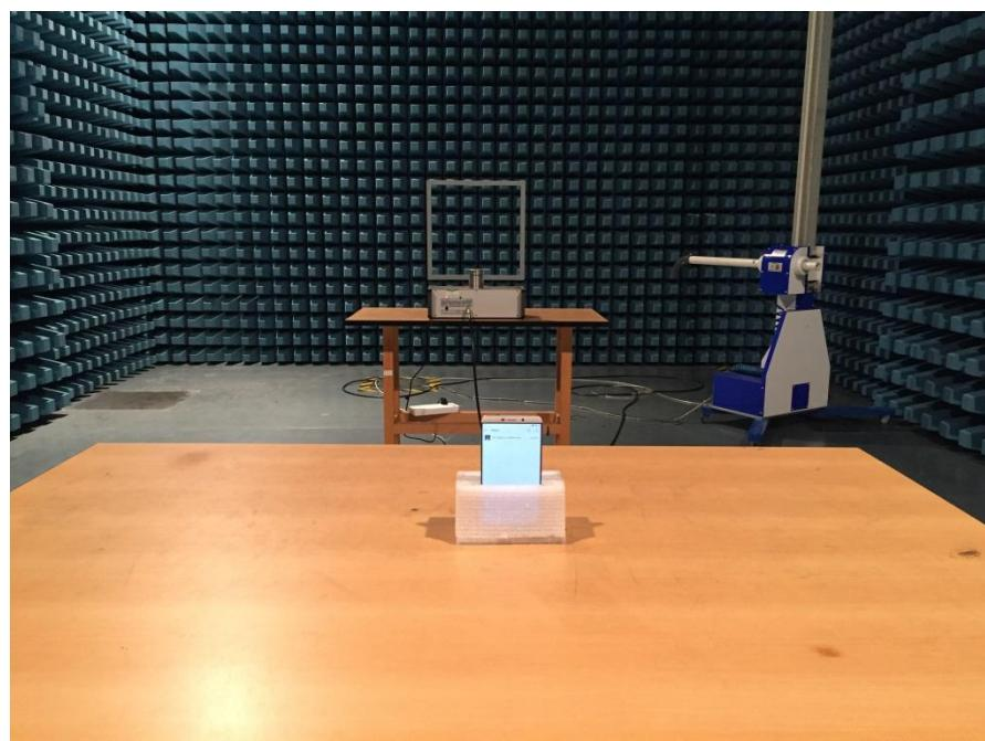
FCC Part15C Radiated Emission 30MHz-1GHZ
