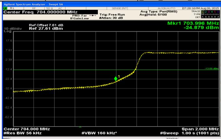
(Channel Bandwidth: 5 MHz)\_LCH\_16QAM\_12RB#6
