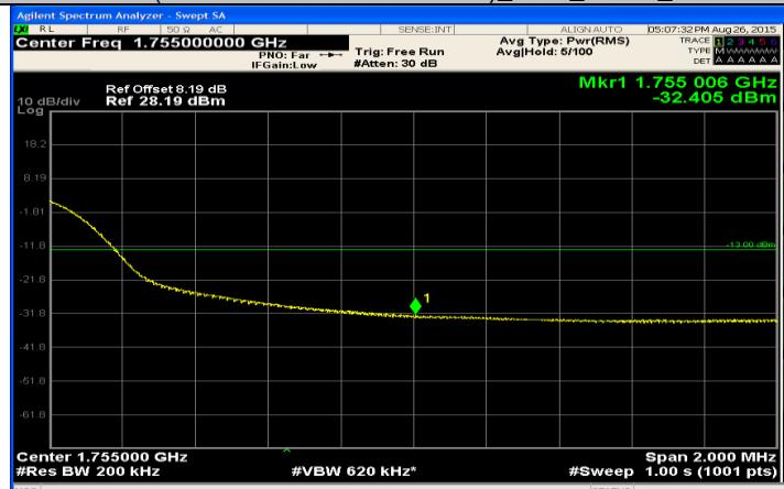
(Channel Bandwidth:20 MHz)\_HCH\_QPSK\_100RB#0
