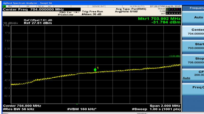
(Channel Bandwidth: 5 MHz)\_LCH\_16QAM\_12RB#13
