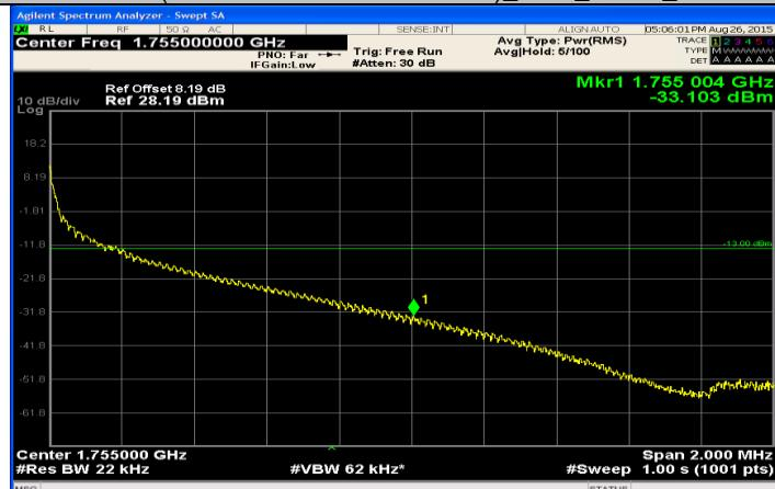
(Channel Bandwidth:20 MHz)\_HCH\_QPSK\_50RB#0
