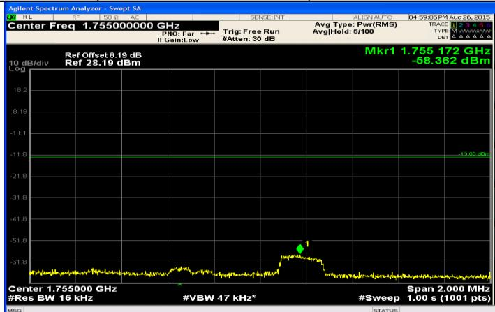
(Channel Bandwidth:15 MHz)\_HCH\_16QAM\_1RB#74
