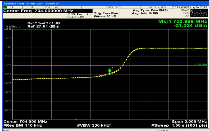
(Channel Bandwidth: 5 MHz)\_HCH\_QPSK\_1RB#0
