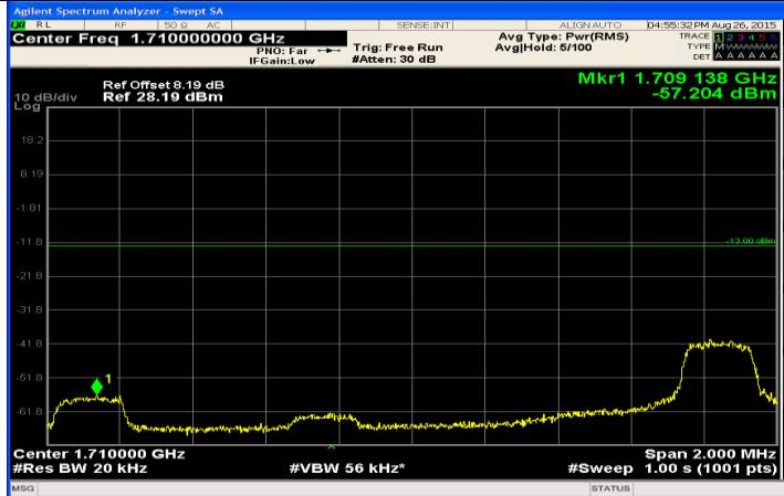
(Channel Bandwidth:15 MHz)\_LCH\_16QAM\_37RB#0
