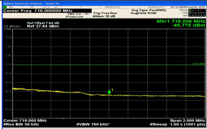
(Channel Bandwidth: 5 MHz)\_HCH\_16QAM\_12RB#6
