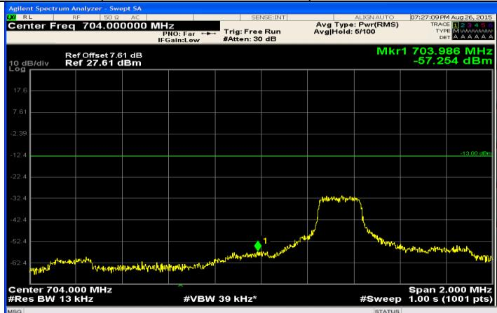
(Channel Bandwidth: 5 MHz)\_LCH\_16QAM\_12RB#0
