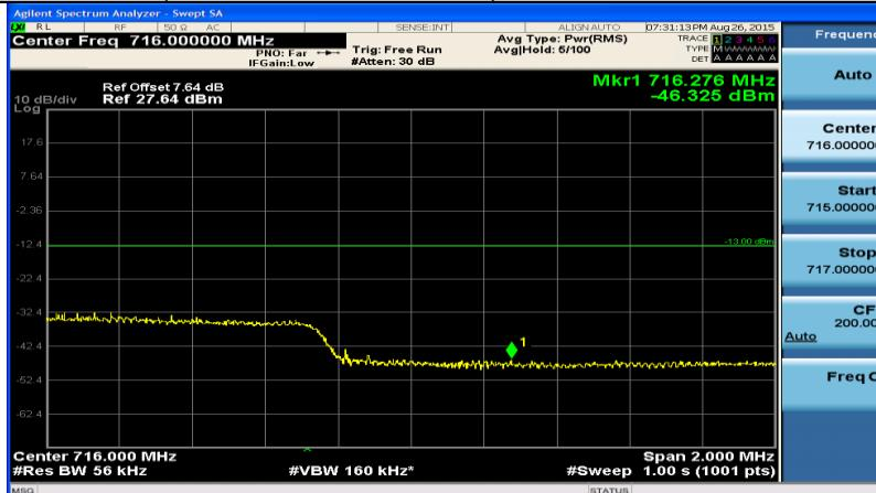
(Channel Bandwidth: 5 MHz)\_HCH\_QPSK\_12RB#6
