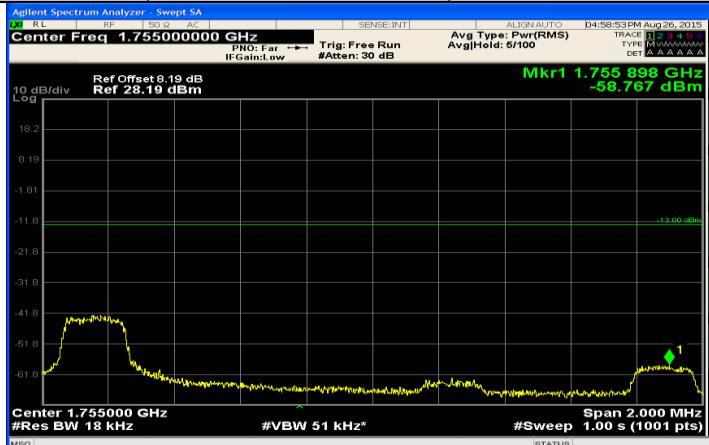
(Channel Bandwidth:15 MHz)\_HCH\_16QAM\_1RB#37
