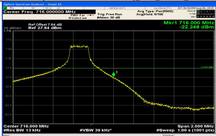
(Channel Bandwidth: 5 MHz)\_HCH\_16QAM\_12RB#0
