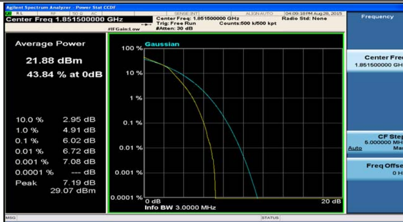
(Channel Bandwidth: 3 MHz)_MCH_16QAM_1RB#0
