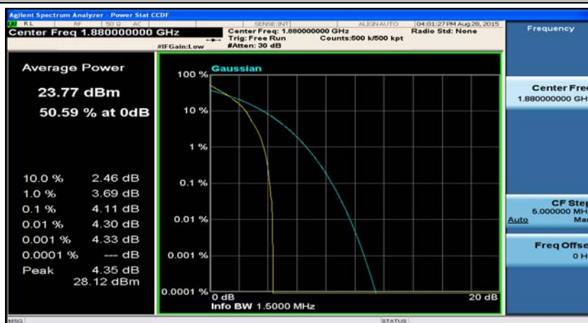
(Channel Bandwidth: 1.4 MHz)_MCH_QPSK_1RB#3
