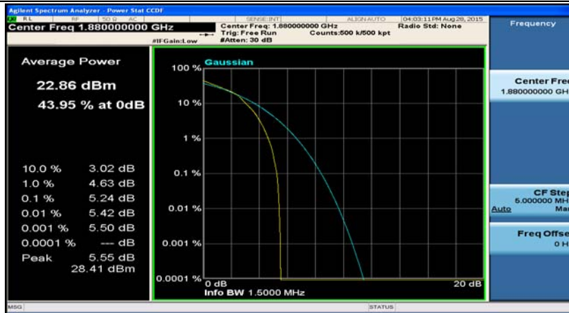
(Channel Bandwidth: 1.4 MHz)_MCH_16QAM_6RB#0
