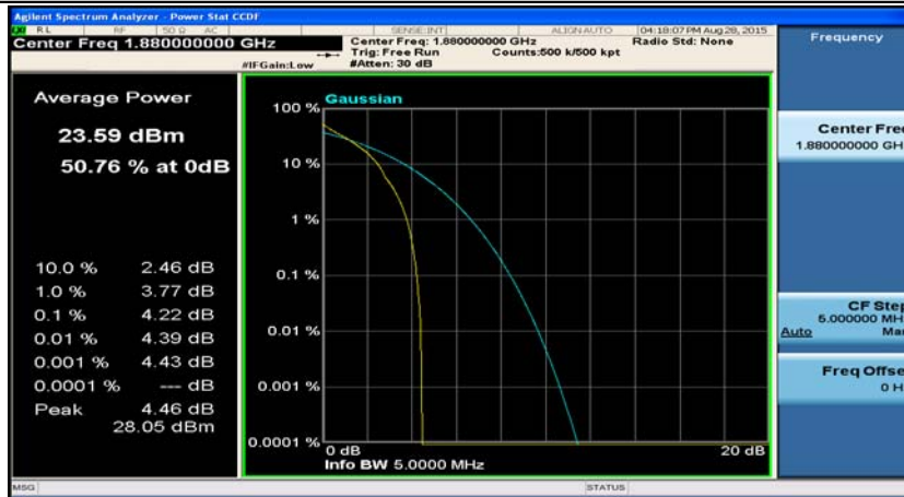
(Channel Bandwidth: 5 MHz)_MCH_QPSK_12RB#0
