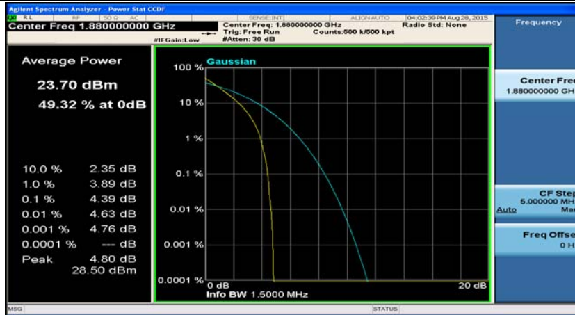
(Channel Bandwidth: 1.4 MHz)_MCH_QPSK_6RB#0
