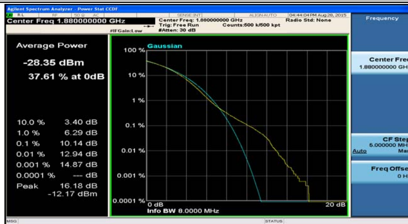
(Channel Bandwidth: 20 MHz)_MCH_QPSK_1RB#49
