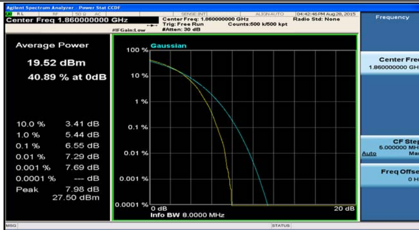
(Channel Bandwidth: 20 MHz)_LCH_16QAM_50RB#25
