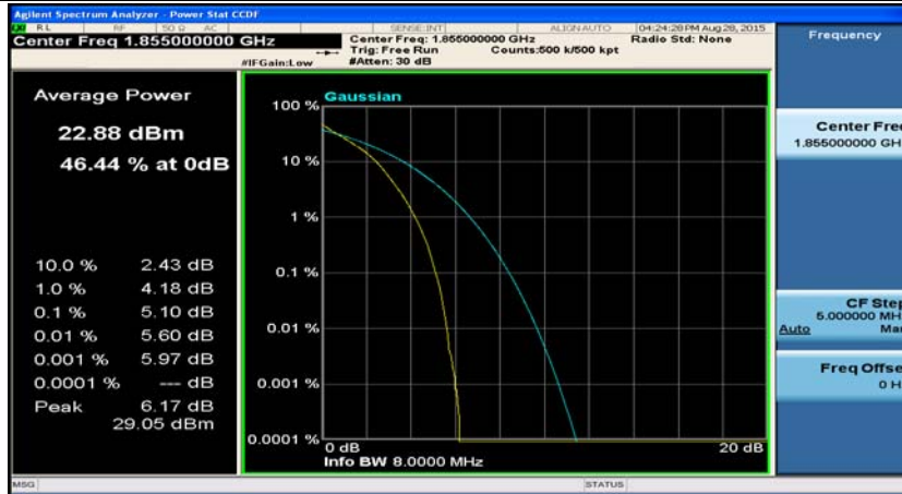
Channel Bandwidth: 10 MHz_LCH_QPSK_25RB#12
