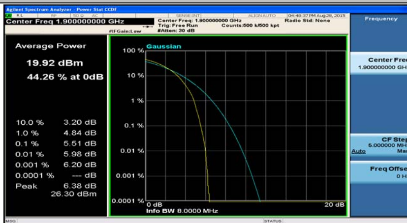
(Channel Bandwidth: 20 MHz)_HCH_QPSK_50RB#0
