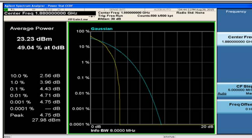
(Channel Bandwidth: 20 MHz)_MCH_QPSK_1RB#49
