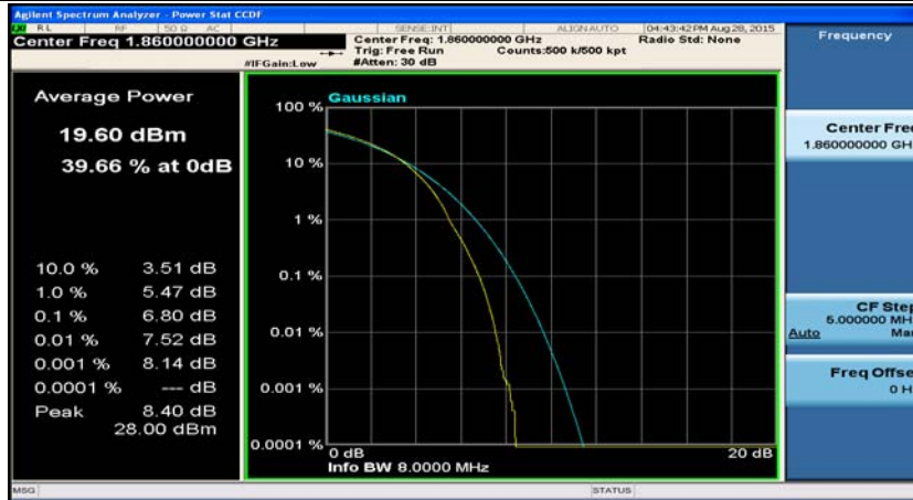
(Channel Bandwidth: 20 MHz)_MCH_16QAM_1RB#0
