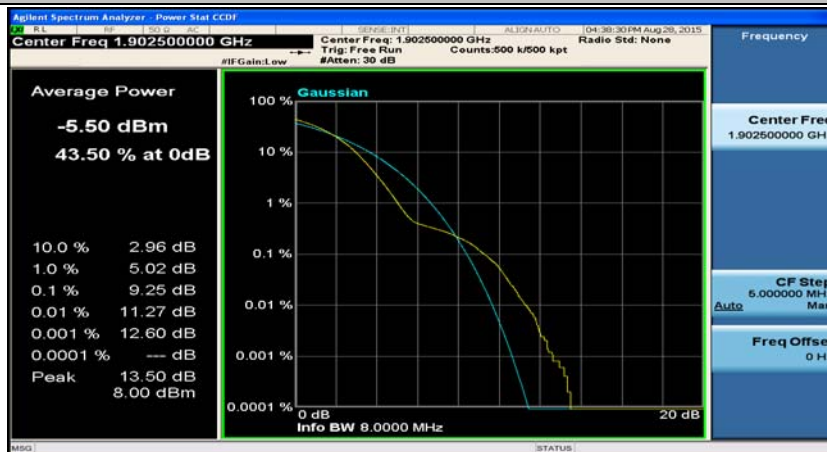
(Channel Bandwidth: 15 MHz)_HCH_16QAM_1RB#0
