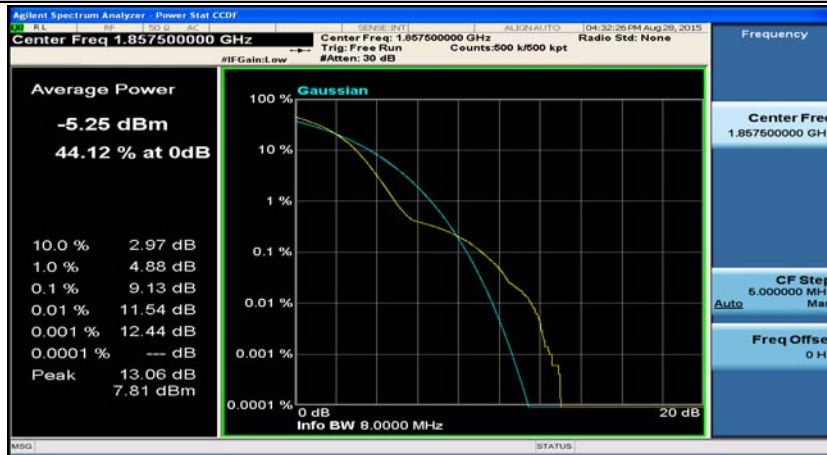
(Channel Bandwidth: 15 MHz)_LCH_16QAM_1RB#37
