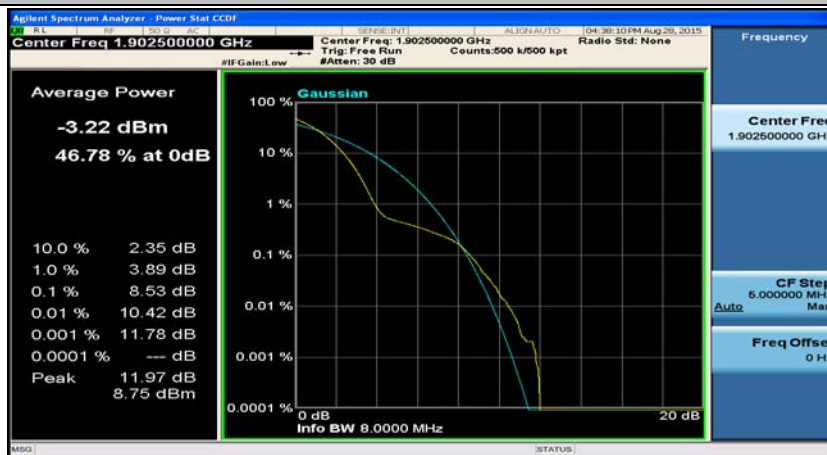
(Channel Bandwidth: 15 MHz)_HCH_QPSK_37RB#0
