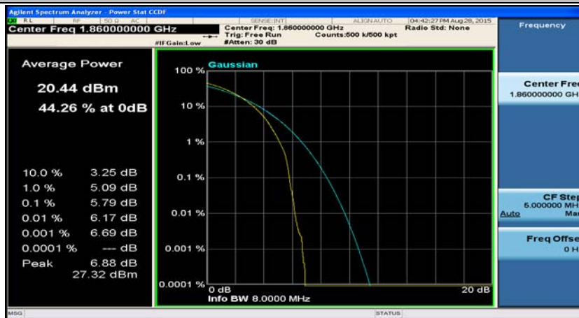
(Channel Bandwidth: 20 MHz)_LCH_QPSK_50RB#50
