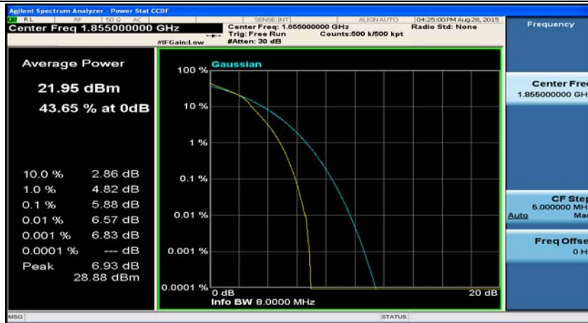
Channel Bandwidth: 10 MHz_LCH_16QAM_25RB#12
