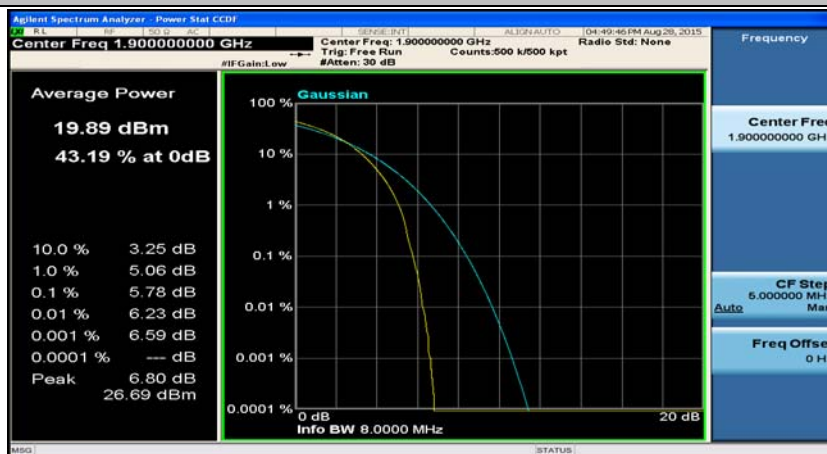
(Channel Bandwidth: 20 MHz)_HCH_QPSK_100RB#0
