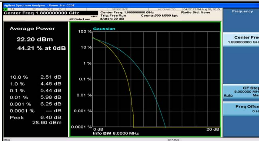
Channel Bandwidth: 10 MHz_MCH_QPSK_25RB#12
