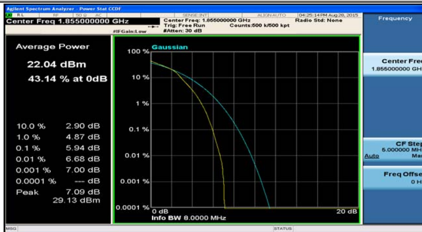
Channel Bandwidth: 10 MHz_LCH_16QAM_25RB#25
