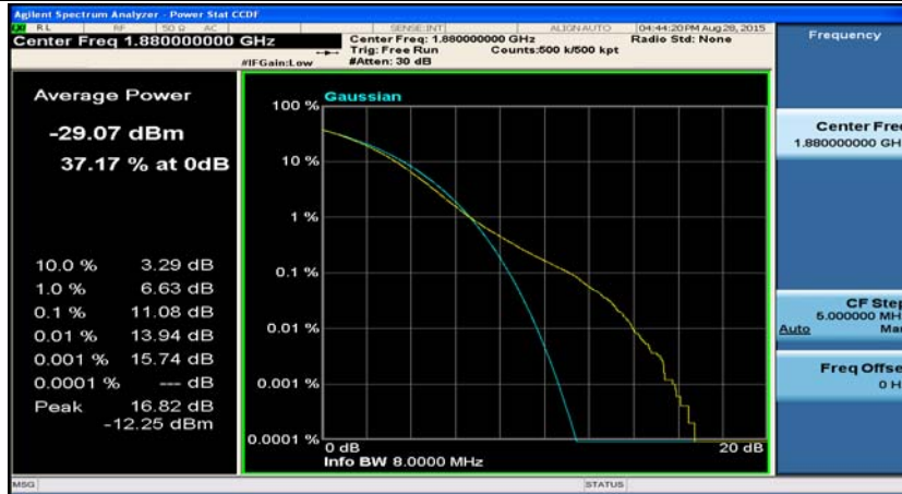
(Channel Bandwidth: 20 MHz)_MCH_QPSK_50RB#0
