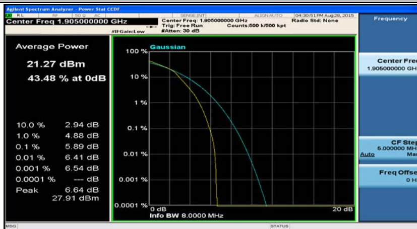
Channel Bandwidth: 10 MHz_HCH_16QAM_50RB#0
