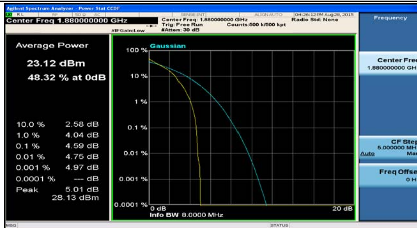
Channel Bandwidth: 10 MHz_MCH_QPSK_1RB#24
