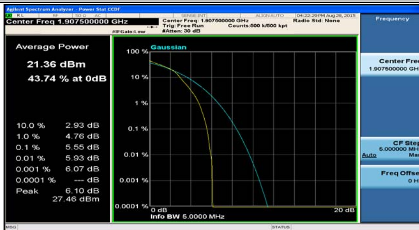
(Channel Bandwidth: 5 MHz)_HCH_16QAM_25RB#0
