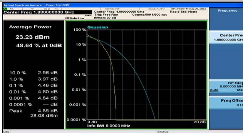
(Channel Bandwidth: 15 MHz)_MCH_QPSK_1RB#37
