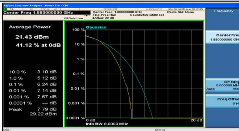
(Channel Bandwidth: 15 MHz)_MCH_16QAM_37RB#18
