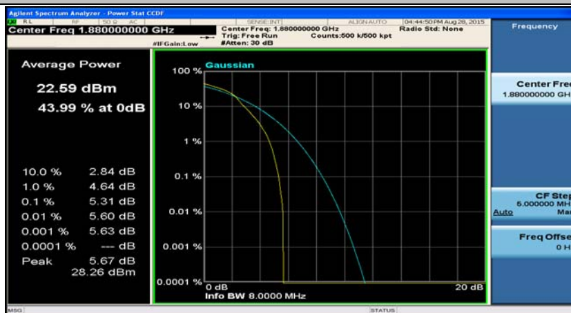
(Channel Bandwidth: 20 MHz)_MCH_16QAM_1RB#49
