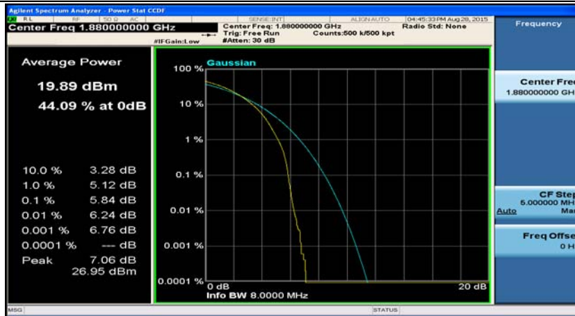
(Channel Bandwidth: 20 MHz)_MCH_QPSK_100RB#0
