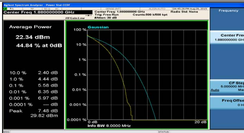
(Channel Bandwidth: 20 MHz)_MCH_QPSK_50RB#25
