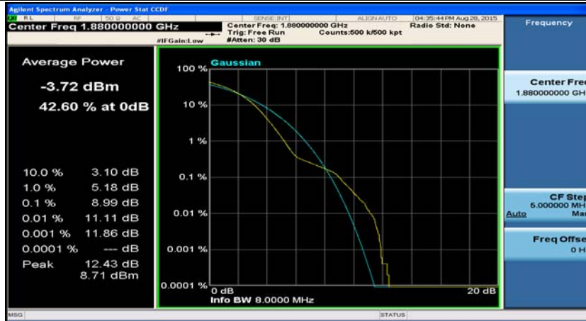
(Channel Bandwidth: 15 MHz)_MCH_16QAM_37RB#0
